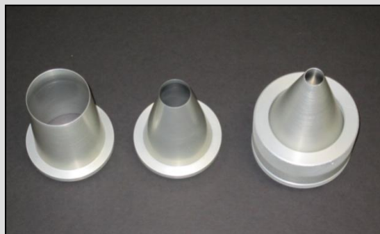
Isokinetic nozzles (114 Lpm, 90 mm filter) designed for determination of reference concentrations
