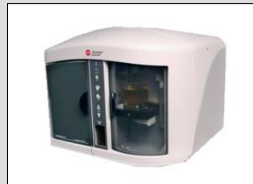
Multisizer IV Coulter Counter used for measuring the concentration and size distribution of collected test aerosols
