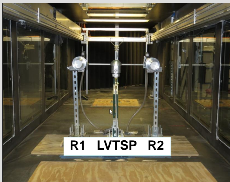
Isokinetic nozzles (114 Lpm, 90 mm filter) designed for determination of reference concentrations
