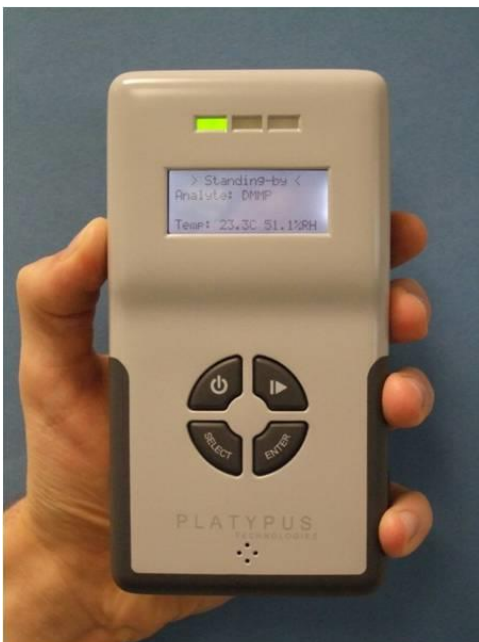
Platypus prototype handheld NO 2 monitor
