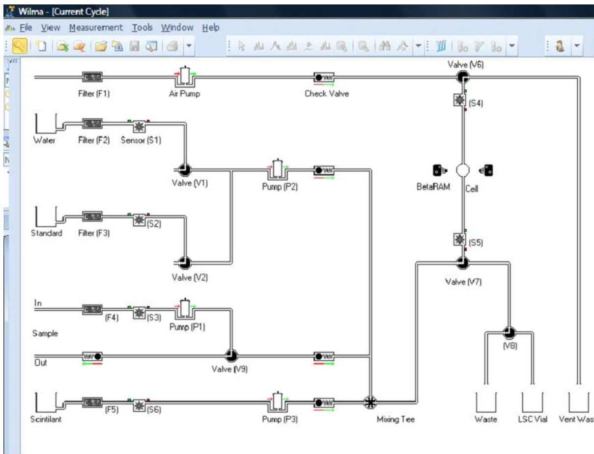
**Figure 2. Flow paths in Walter unit and the  $\beta$ -RAM system.**
