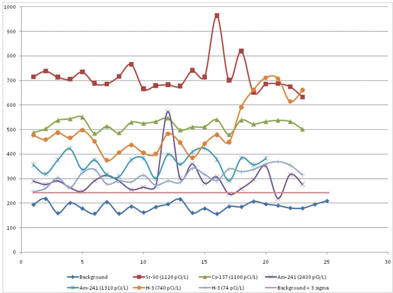
**Figure 6. Overall Summary of  $\beta$ -RAM system testing. Counts (y-axis) versus test runs**
