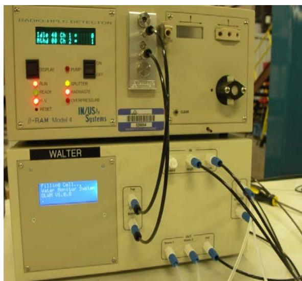
**Figure 1. Model 4 β-RAM scintillation-counting system and Walter fluid handling/distribution unit.**
