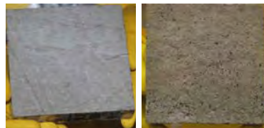
Coupons before/after grit blast
