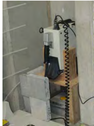
ORTEC portable high purity germanium detector counting Cs-137 gamma radiation on a concrete coupon
