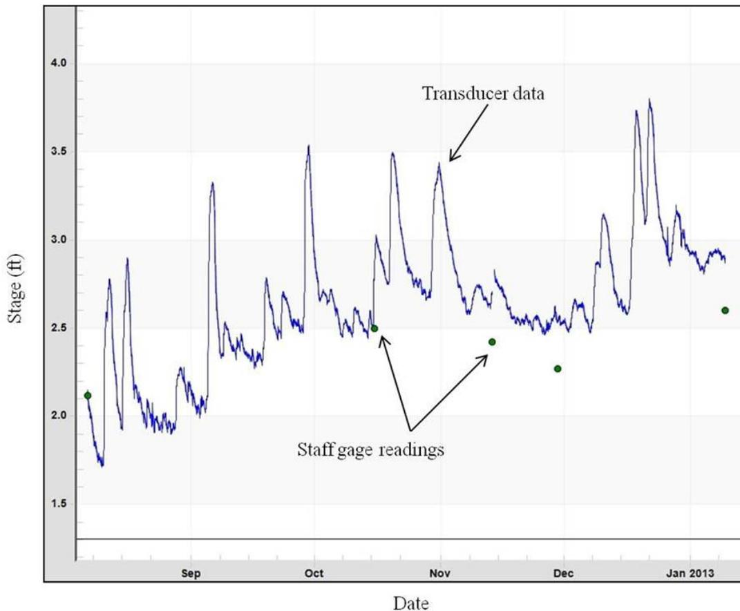
Figure 16. Staff gage readings provide a quality check of transducer data. In this example, staff gage readings stopped matching transducer readings in November, indicating that the transducer or gage may have changed elevation.
