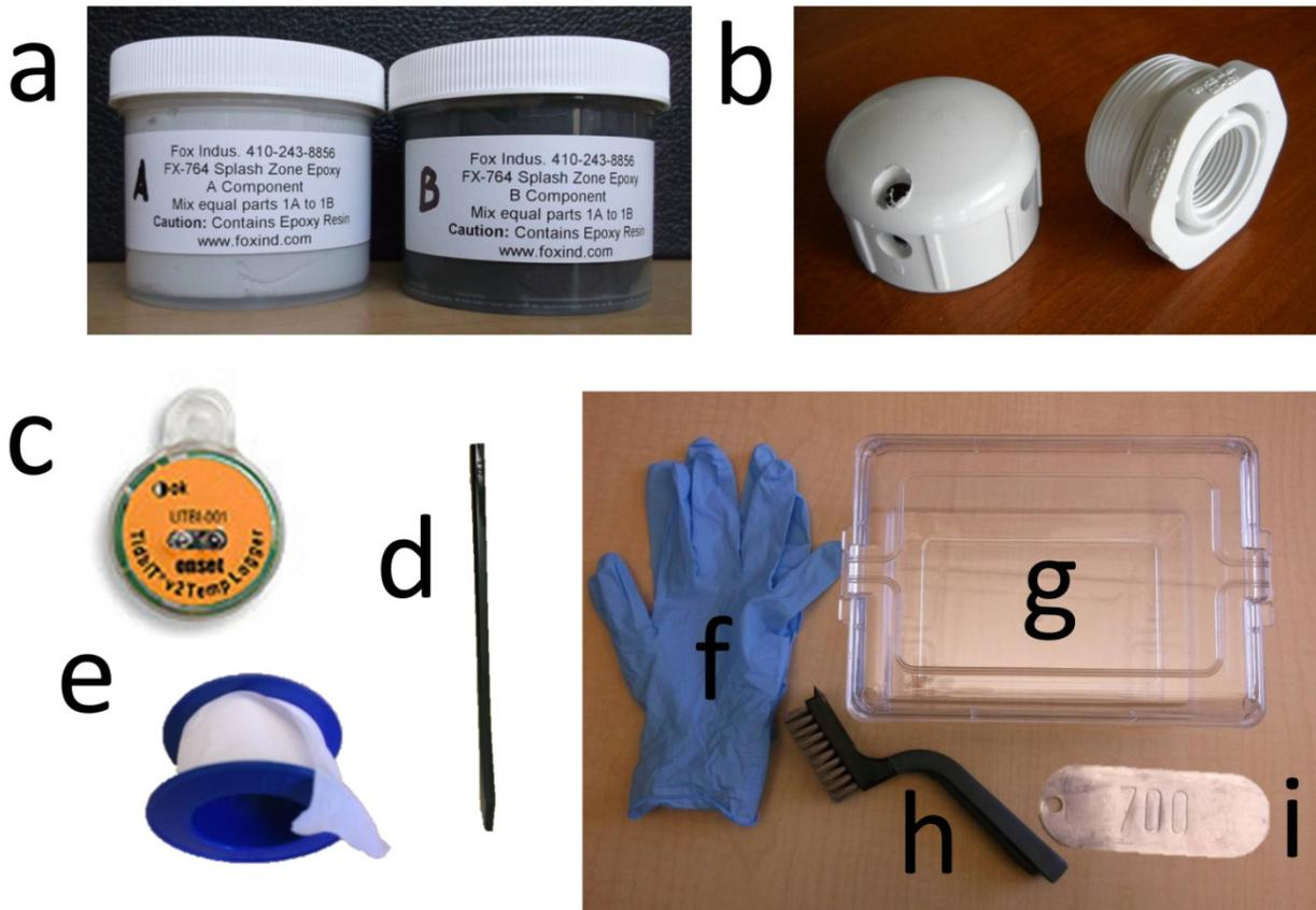
Figure 9. Equipment needed to permanently install temperature sensors in streams using underwater epoxy includes: (a) two-part FX-764 epoxy from Fox Industries, (b) PVC solar shield, (c) temperature sensor, (d) cable ties, (e) plumber's tape, (f) rubber gloves, and (g) plastic viewing box, (h) wire brush, and (i) metal forestry tree tag (Isaak and Horan 2013).
