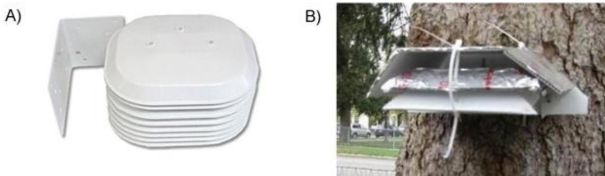
Figure 5. Examples of radiation shields for air temperature sensors include A) the Gill-style Onset RS1 solar radiation shield ([www.onsetcomp.com](http://www.onsetcomp.com)) and B) custom design by Zachary Holden (Appendix B).
