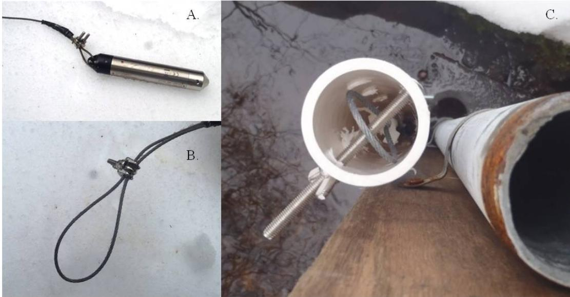
**Figure 20. Non-vented pressure transducer installation. A. Non-stretch cable is attached to transducer, B. Loop is made at non-transducer end of cable, C. Cable with transducer is suspended over bolt from top of PVC pipe.**
