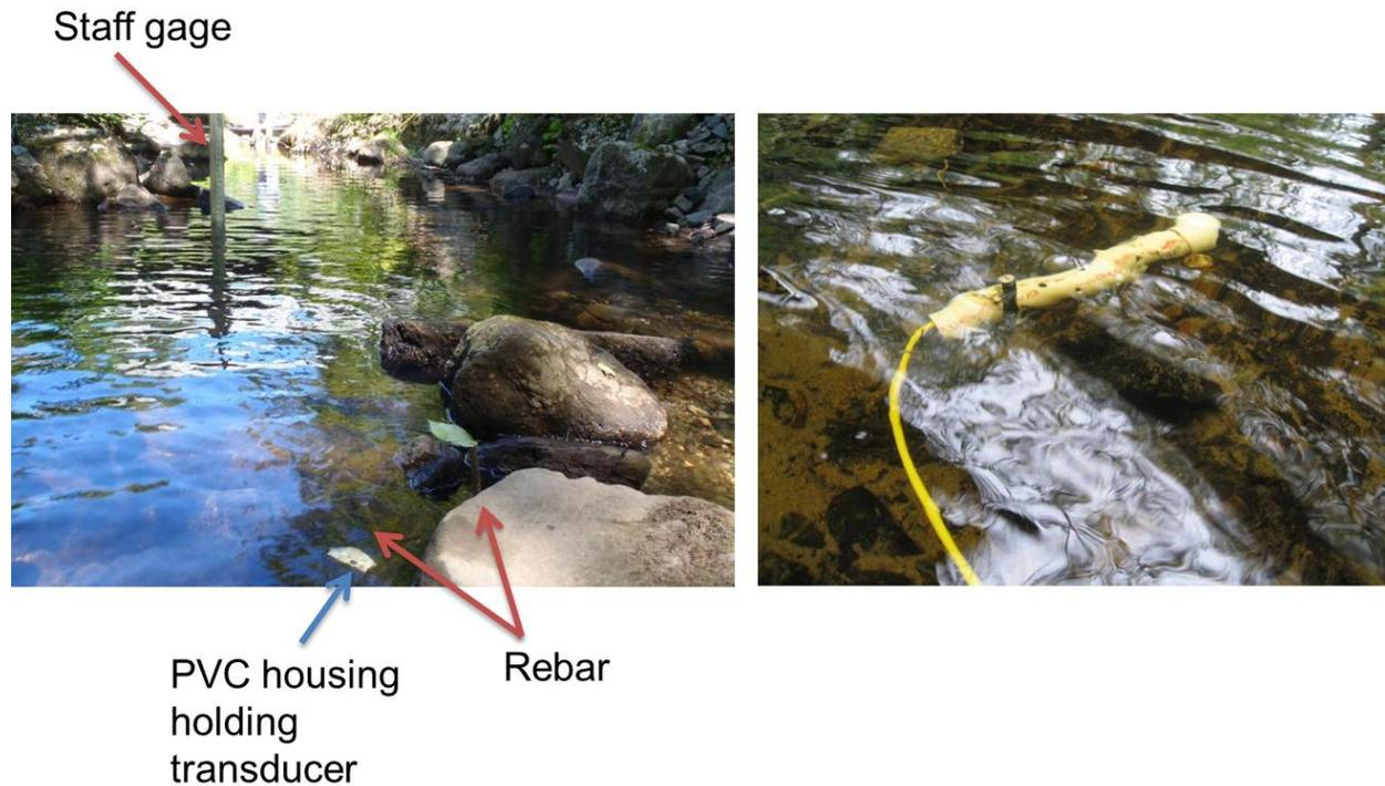
Figure 22. Examples of streambed installations of pressure transducers using rebar.
