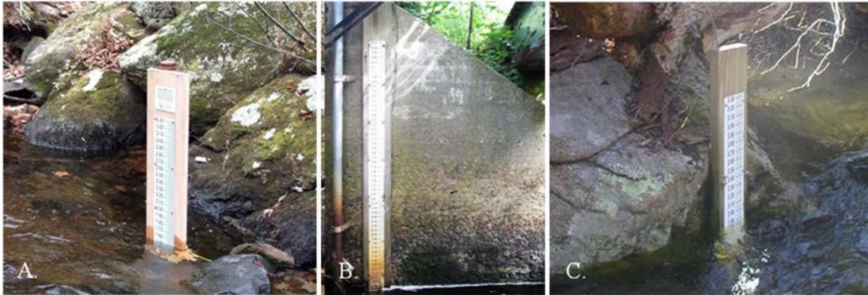
Figure 18. Examples of gage installation techniques include, A. streambed, B. fixed object (bridge wing wall) and C. fixed object (boulder).
