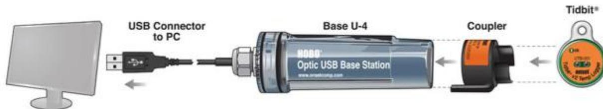
Figure 2. Additional equipment is needed to offload data from the temperature sensors onto a computer. This figure depicts the coupler, base station, and USB cable that are needed to download data from the Onset Tidbit® v2 sensor ([www.onsetcomp.com](http://www.onsetcomp.com)). A waterproof shuttle can also be used in place of the base station for on-site data offload and temporary data storage. These devices must be compatible with the make and model of the sensor.
