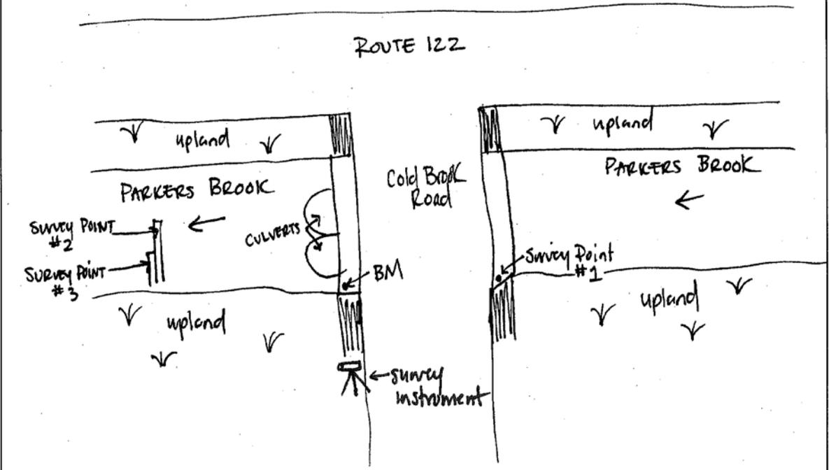
Figure 26. An example of a completed elevation survey form.
