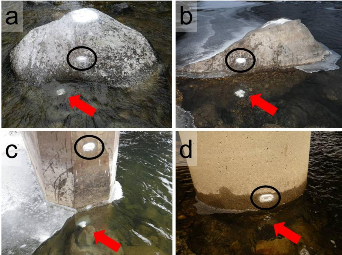
Figure 7. Examples of large rocks (a and b) and cement bridge pilings (c and d) that provide good sensor attachment sites. Each site has a flat downstream attachment surface that is shielded during floods from bedload and debris. Arrows point to the solar shield containing a sensor; circles highlight metal forestry tags epoxied above the sensor to monument the site (photos taken from Isaak et al. 2013).
