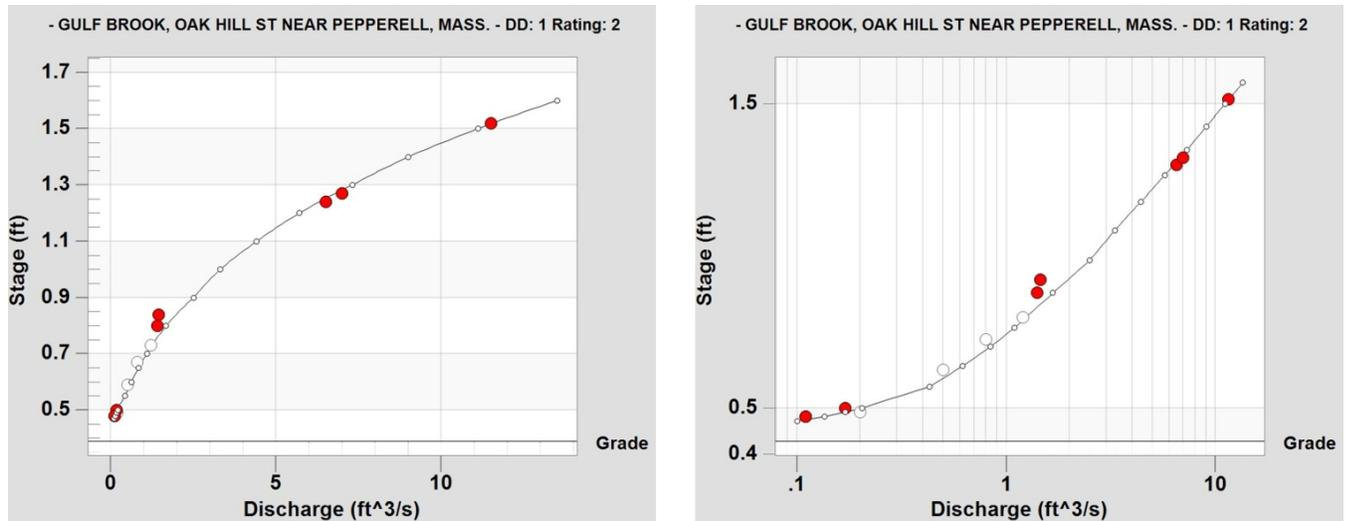
Figure 32. Example of regular (left) and log-log scale (right) rating curves created using Aquatic Informatics' AQUARIUS software.
