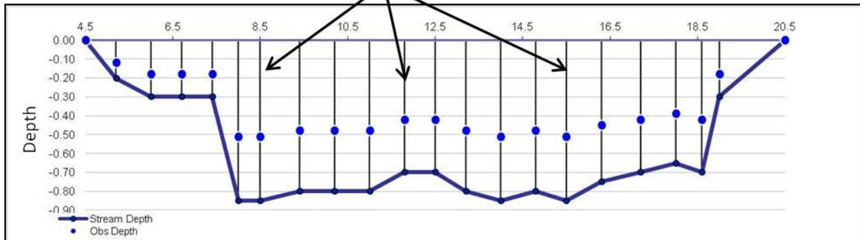
Figure 31. Layout of a channel cross-section for obtaining discharge data, using the velocity-area procedure.
