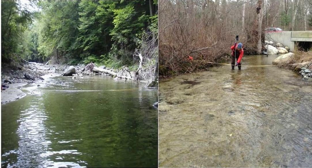
Figure 30. Examples of good cross-sections for making discharge measurements.
