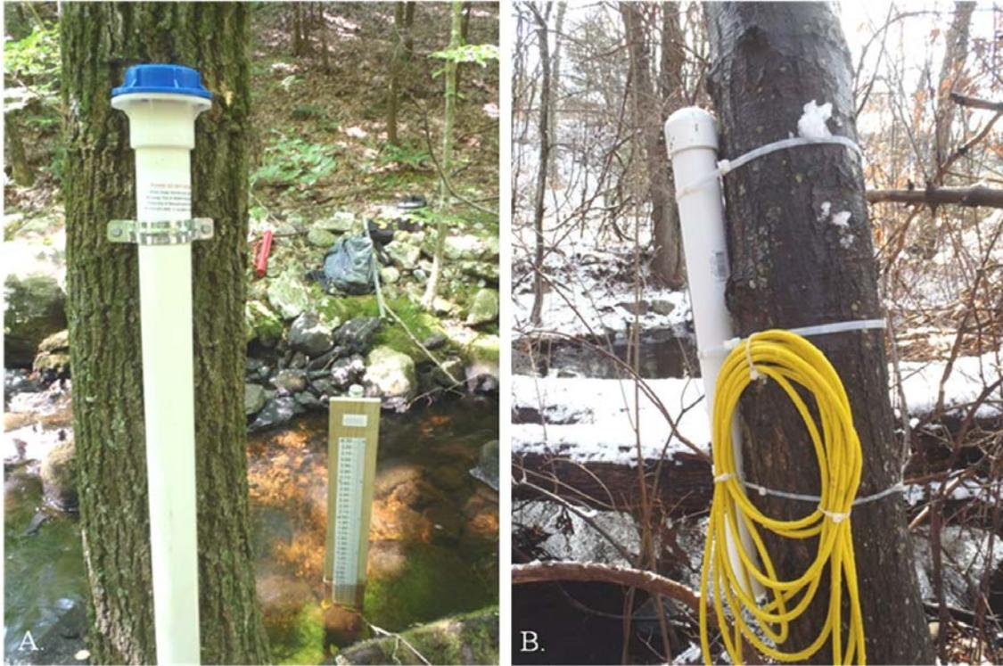
Figure 23. Vented transducer data logger installation using A. stainless steel conduit straps and B. cable ties.
