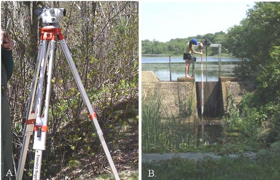
Figure 25. Example of auto level and tripod used for elevation survey (A) and of a permanent structure used as a benchmark (B).
