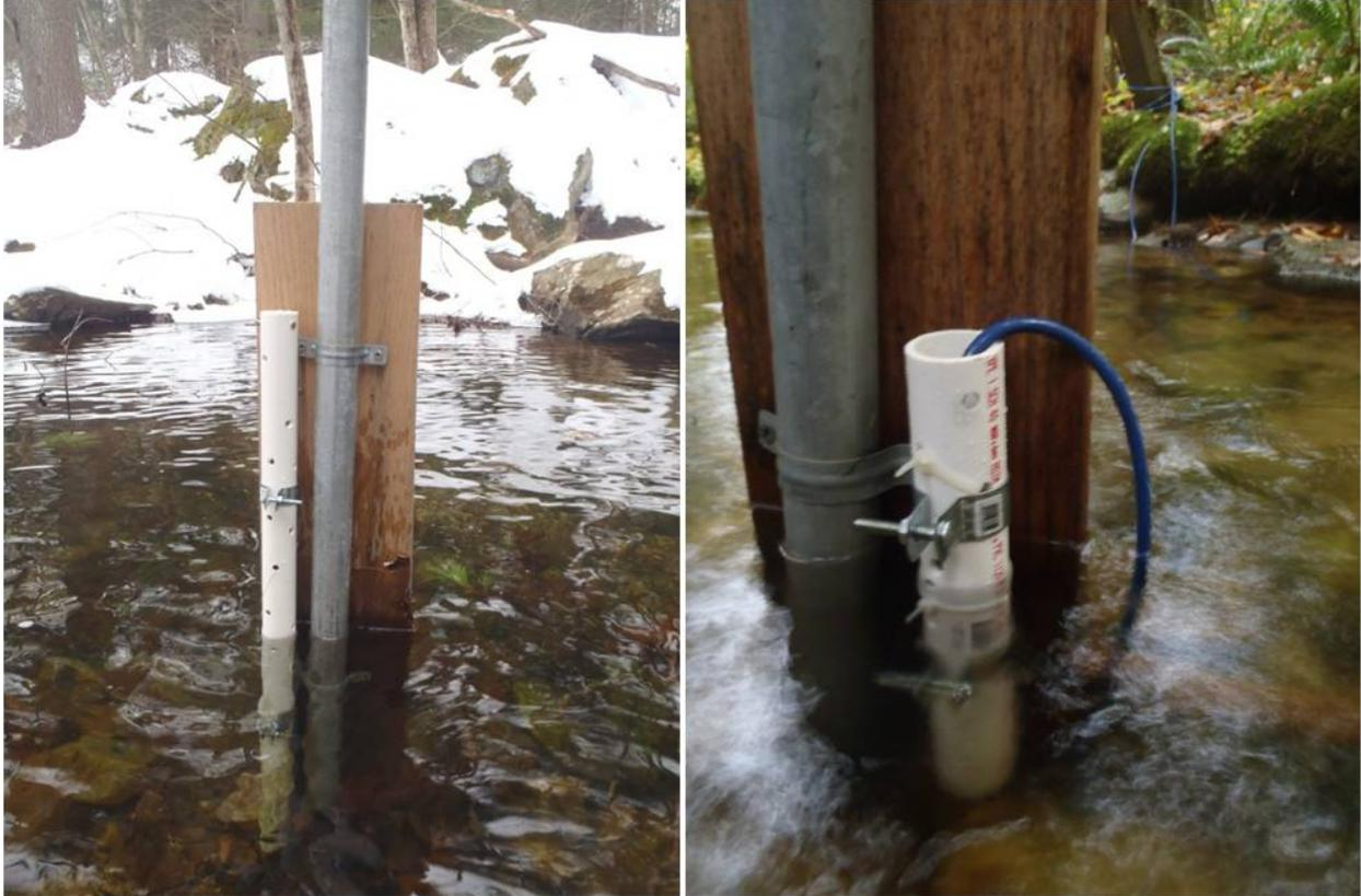
**Figure 21. Non-vented (left) and vented (right) pressure transducers attached to staff gage board using conduit hangars.**
