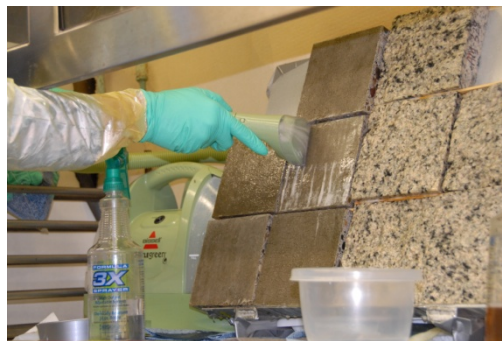
Figure 3-4. Rinsing and vacuuming RRII from concrete coupon
