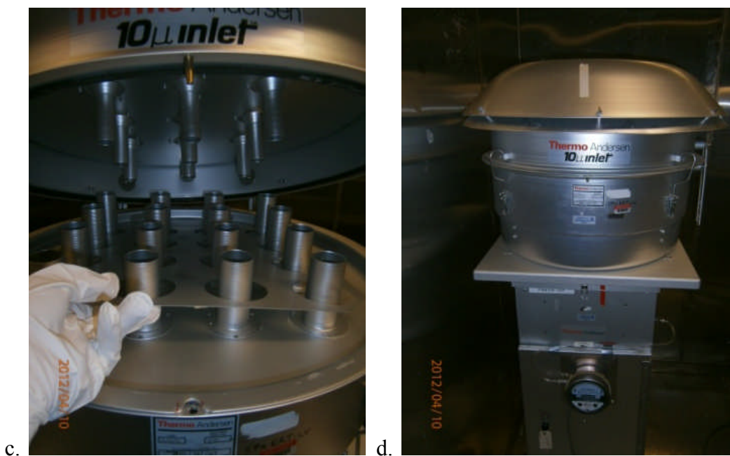
Figure 2. a) HiVol sampler with head unit and top open, and filter vent secured; b) head unit closed and latched; c) placement of shim; and d) top closed and latched.
