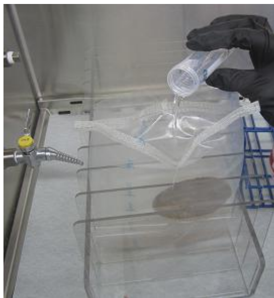
Figure 7. Pouring remainder of 90 mL PBST into stomacher bag.
