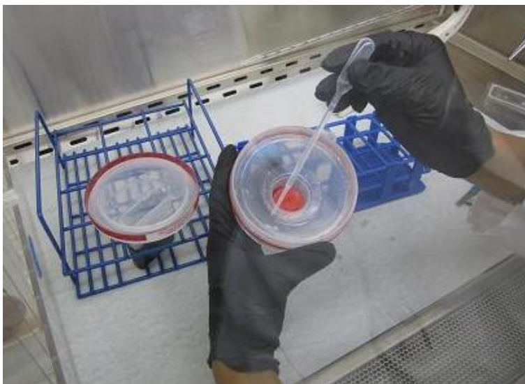
Figure 6. Rinsing inside walls of filter case.
