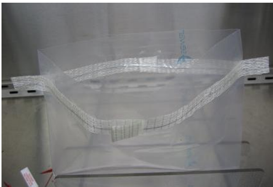
Figure 3. Stomacher bag in bag holder with wires in open position, ready to accept filter and liquid.
