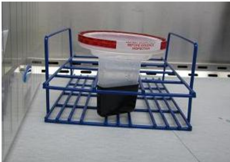
Figure 2. Place the top half of the filter case onto a rack so that the filter can be removed from the bottom half of the filter case.
