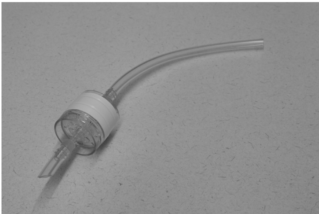
Figure 2-6. Filter (37 mm) Cassette with Nozzle and Tubing
