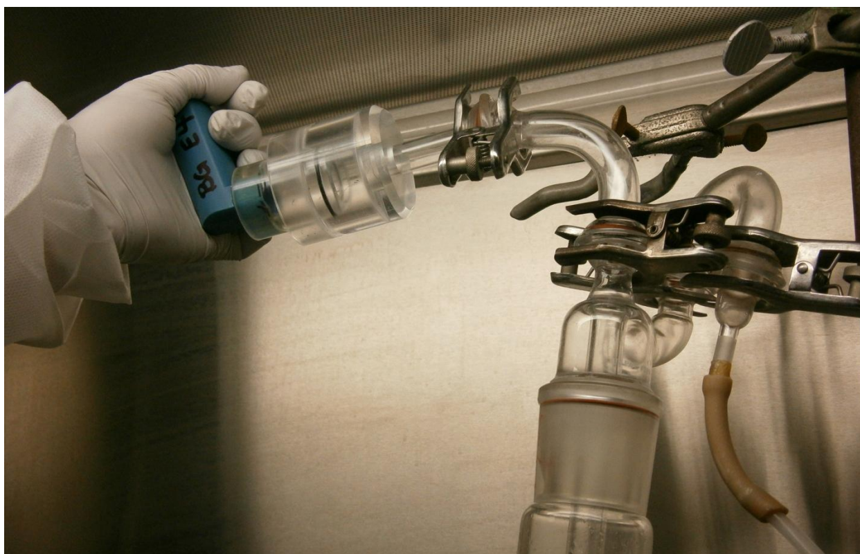
Figure 1. MDI orientation while dispensing test puffs into the aerosol trap.
