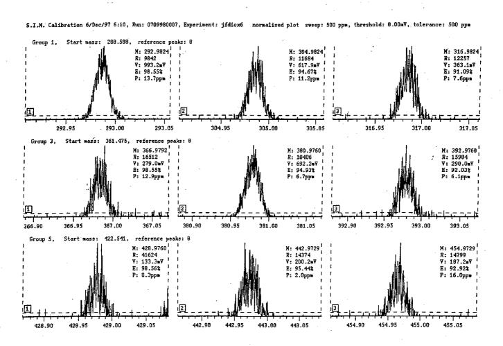
Figure 8-2 Resolution/Mass Calibration for MS
