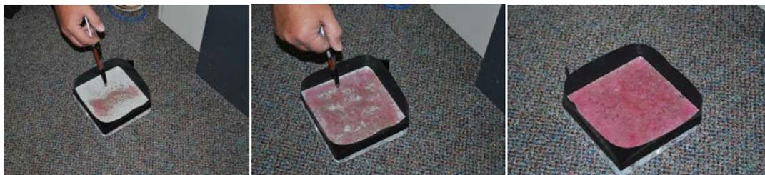
**Figure 3-1. Demonstration of contaminant application technique.**
