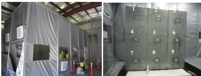
**Figure 3-2. Containment tent (outer view) and inner view with test stand containing contaminated coupons.**
