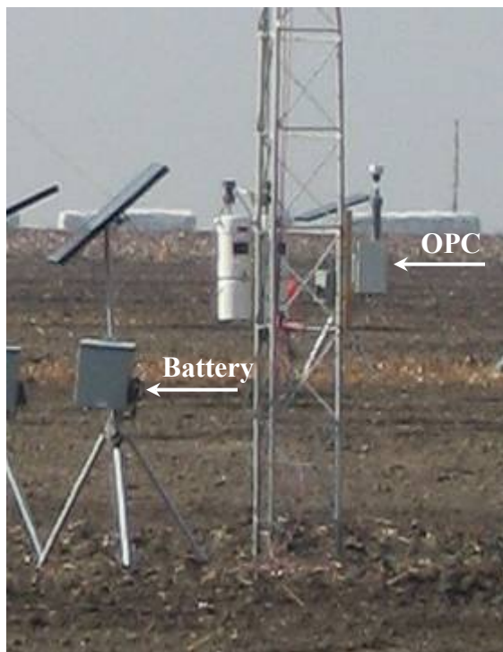
Figure 11. Met One Instruments Optical Particle Counter (OPC) Model 9722, indicated by arrow, setup for field deployment on a tower base with an accompanying rechargeable battery pack and solar panel.
