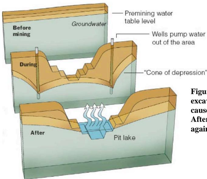
**Figure 6. Illustration of how pumping water from an excavation as occurs during mining during mining can cause a cone of depression in the surrounding water table. After mining ceases, pumping stops and the excavation fills again but remains lower due to evaporation.**
