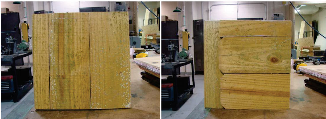
Figure 2-3. Rough-Cut Barn Wood Coupon Front (Left) and Back (Right) (Note Offset of Wood Orientation)
