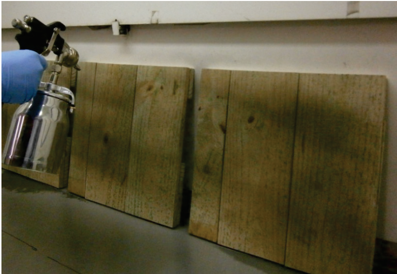
Figure 2-5. Application of Grime to Coupons
