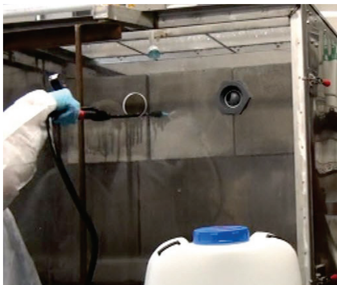
Figure 2-7. Spraying Through Center-Aligned Port in the Small Chamber Door
