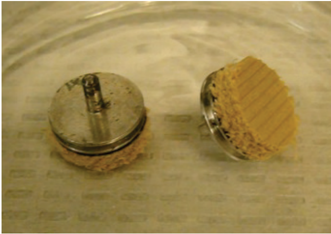
Figure 2-1. 18 mm Rough-Cut Barn Wood Coupon (Task 1)
