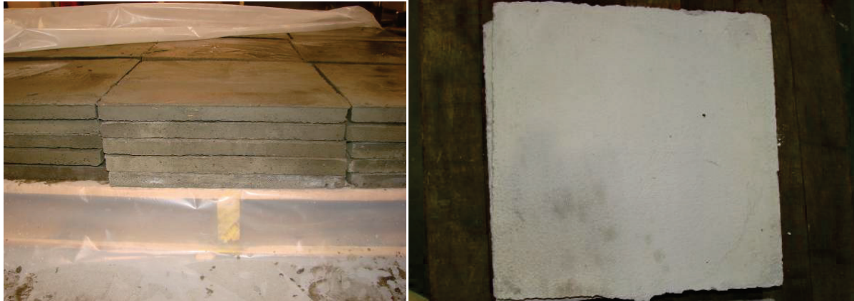
Figure 2-4. Curing Concrete (Left) and Final Concrete Coupon (Right)
