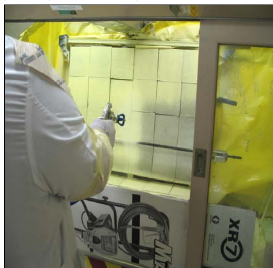
Figure 1. Applying the Coating With a Sprayer
