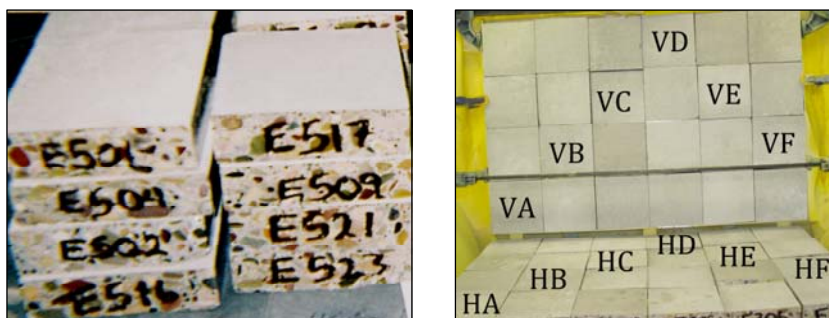
Figure 2. Concrete Coupons (left) and Test Stand With Contaminated Coupons (right) - H is horizontal and V is vertical, A–F indicate the surface positions
