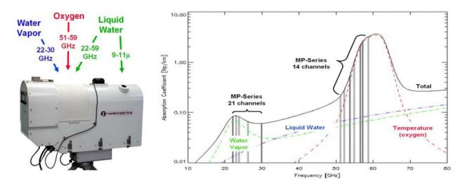
Figure 1-4. The atmospheric emissions spectrum received by a multi-channel radiometer. The microwave spectra are received by various sensors in the radiometer (graphic courtesy of Radiometrics Corporation).
