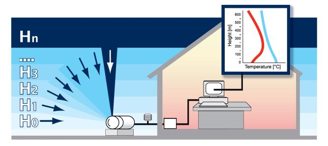
Figure 1-3. Operational technique to obtain a vertical temperature profile (at altitudes  $H_0, H_1 \dots H_n$ ) using the scanning technique. The resulting temperatures represent a volume average at the reported levels (graphic courtesy of Kipp and Zonen).
