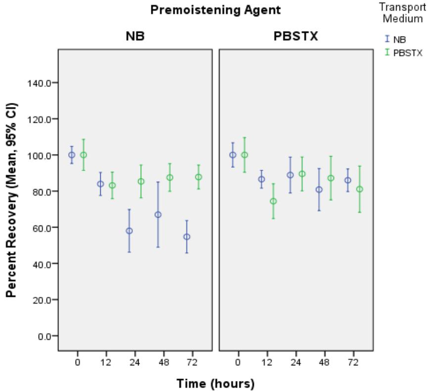
Figure 18: Mean % recovery of *Y. pestis* CO92 ( $10^4$  CFU/ swab) from dirty macrofoam swabs over storage time. Bars represent the 95% confidence interval of the mean recovery (n=10).
