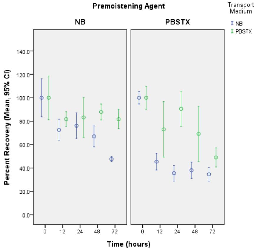
Figure 19: Mean % recovery of *Y. pestis* CO92 ( $10^4$  CFU/ swab) from dirty rayon swabs over storage time. Bars represent the 95% confidence interval of the mean recovery (n=10).
