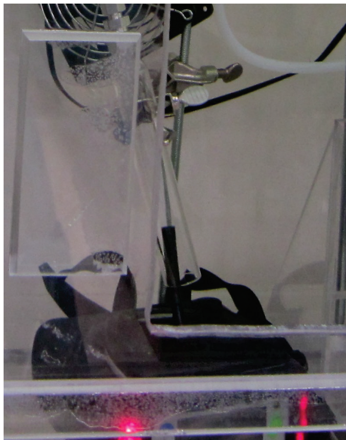
Figure 2.4-3. Example of glass bell tube placed over inlet tube of a detector (Dräger X-am 7000).
