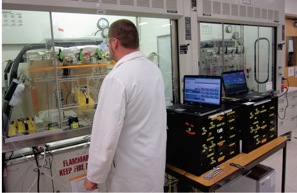
Figure 2.4-2. View of two test systems in adjacent laboratory hoods for testing of handheld detectors.
