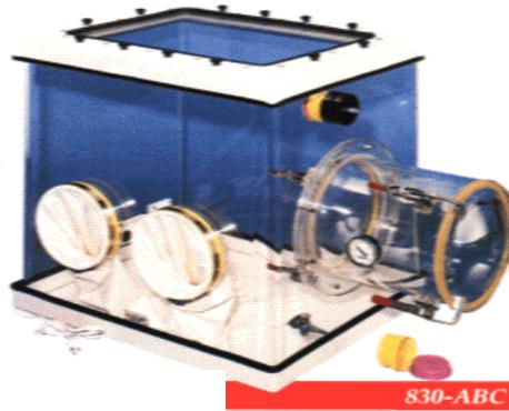
**Figure 2-1. Glove box used for test and control chambers for ClO<sub>2</sub> fumigation testing.**
