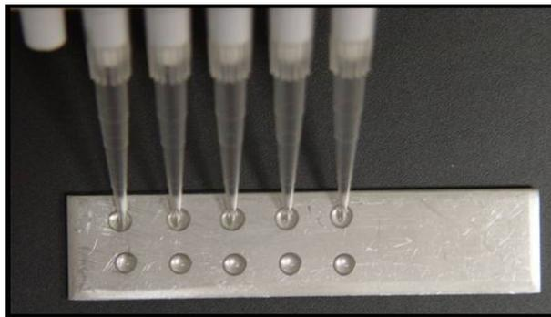
**Figure 2-5. Multichannel micropipette applying biological agent to a coupon.**
