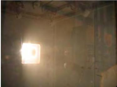
Charged spray of modified DF-200 in the Sandia Aerosol Test Chamber during a cloud knockdown test.
