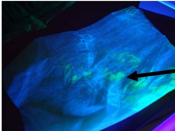
Substantial simulant transfer from surface of car to plastic on untreated side of car
