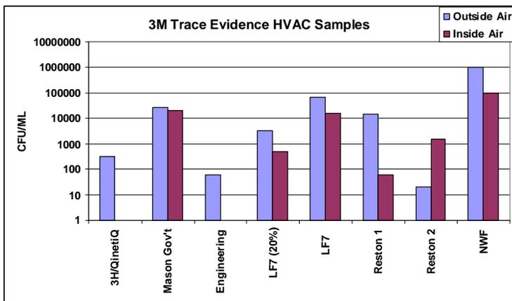
Comparison of inside air side of HVAC filter (concentration in CFU/ML) and outside air concentration of 3M trace evidence samples from buildings (note y-axis logarithmic scale).
