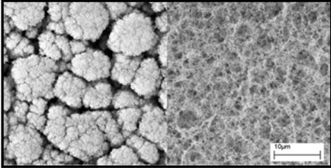
1 nm  $Y_2O_3$  made in 1 Torr  $N_2$       5 nm  $Y_2O_3$  made in 10 Torr  $N_2$
