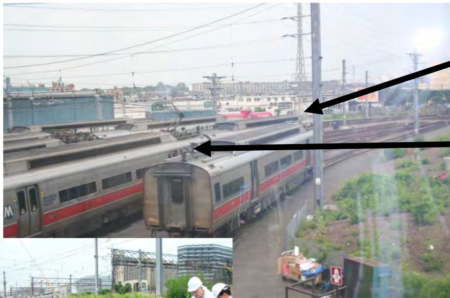
Pantograph down and in locked position
