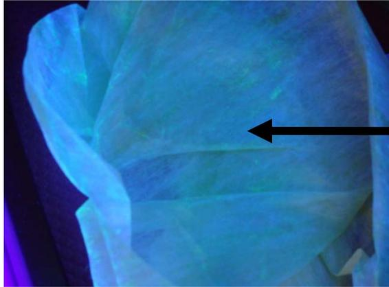
Very little simulant transfer observed on plastic from treated side of car
