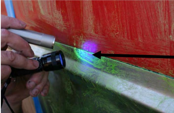
Zone #3 PDT-06 Simulant in interface between painted surface and aluminum after treatment with strip coat
