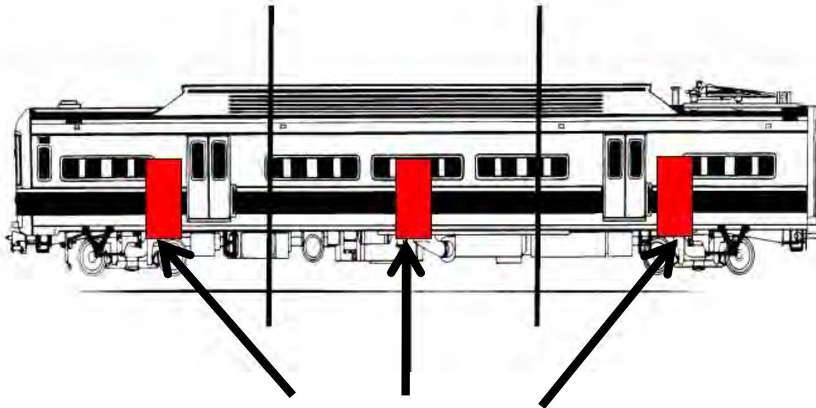
Contamination simulation powder applied to three areas of roughly the same dimension and location as the treated side of car
