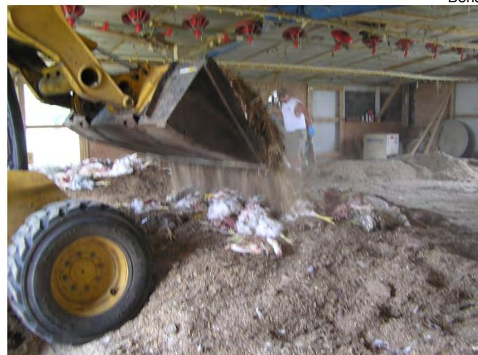
Skid steer loader constructing disposal windrow.
