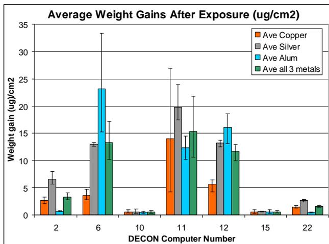
Comparison of Visual Inspection images of the blind test sample with the coupon weight gains enabled Alcatel-Lucent team to identify test conditions corresponding to each PC with 100% accuracy.
