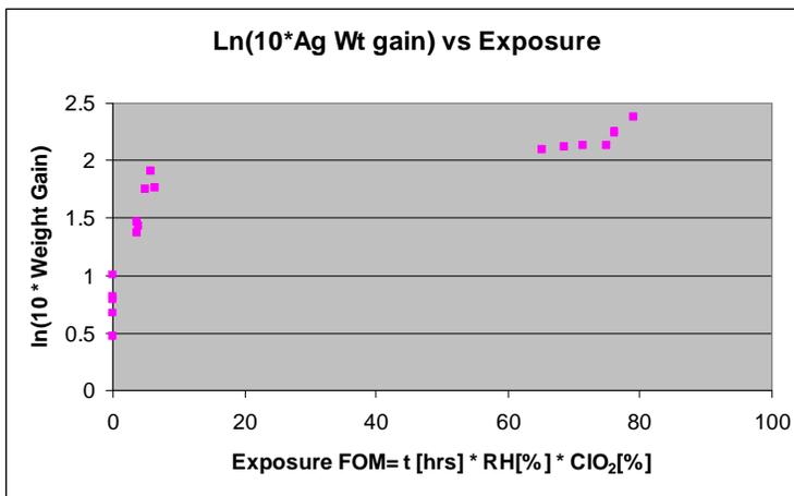
Quantitative data on Corrosion Mass Gain suggests that corrosion is strongly influenced by surface ion transport controlled by adsorption of water. The shape of the curve is similar to a BET Isotherm.
