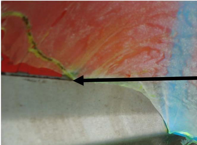
Pretreatment with CC Wet resulted in a complete removal of strip coat (and simulant) from joint in zone 2 without tearing
