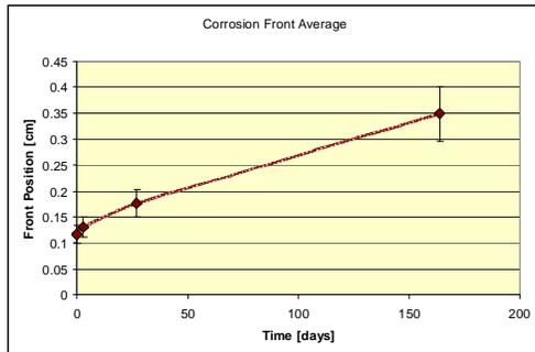
Corrosion Front Progression measured on photographs in slide 18 shows that damage continues for months after initial exposure. Two thirds of damage occurs from weeks to months after the single day decontamination.
