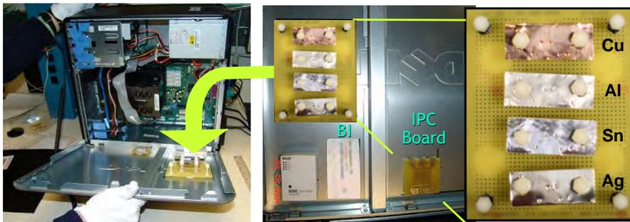
**Quantitative Correlative information** - The use of pure metal coupon process monitors was adapted from ASTM standard<sup>(3)</sup> test methods for calibrating mixed flowing gas test chambers for environmental testing of electronic equipment. The material of the coupons is source-traceable. The effect of each exposure is measured by the weight gain of coupons of Al, Cu, Sn, and Ag using a precision microbalance calibrated using NIST-traceable standards.
