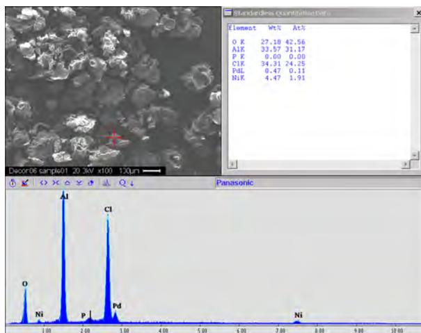
Cl content of corrosion particles emitted by the CPU heat sinks was repeatedly measured over time using Energy-Dispersive X-ray Analysis (EDX).
