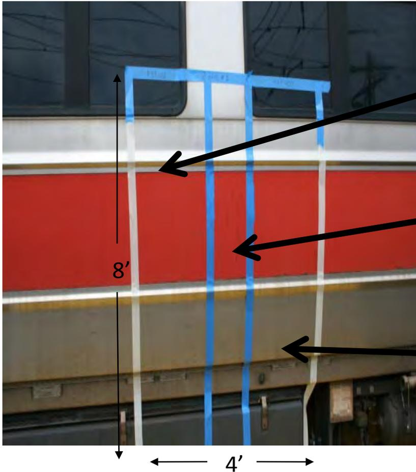
PXT-07 contamination simulant applied
