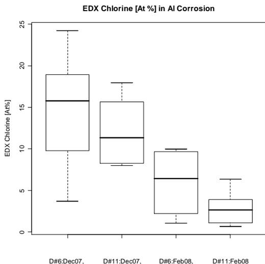
Particles emitted by exposed Aluminum heat sinks change composition through time for months after initial exposure, measured by EDX, as noted on slide 33.
