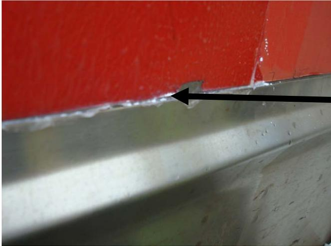
In area without pretreatment (zone 1) a substantial amount of simulant was observed in joint area after removal of stripcoat
