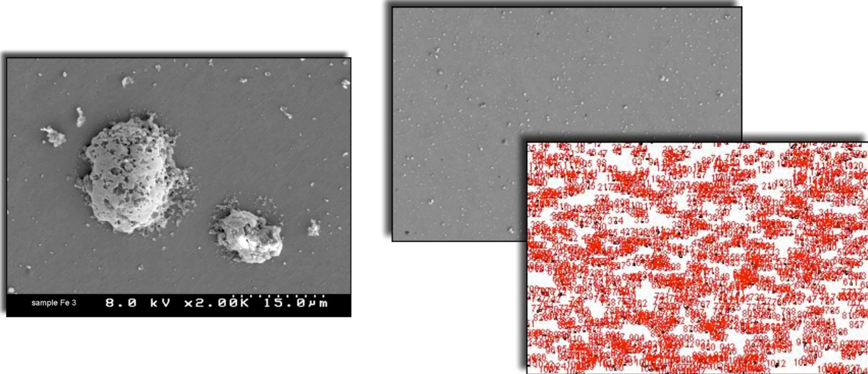
*SEM/EDS images of contaminated surfaces CsCl deposition, particle density, and false color image for particle counting*
