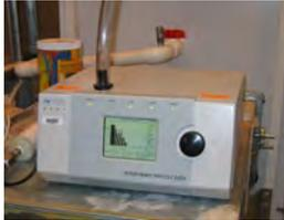
**Aerodynamic Particle Sizer (APS)**
