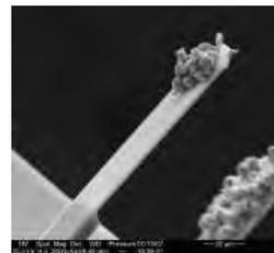
AFM tip with particles adhered
