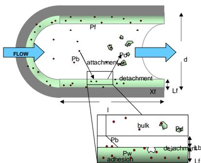
Schematic of pipes showing pipe wall layer where contaminants can adsorb to corrosion products or attach to biofilms
