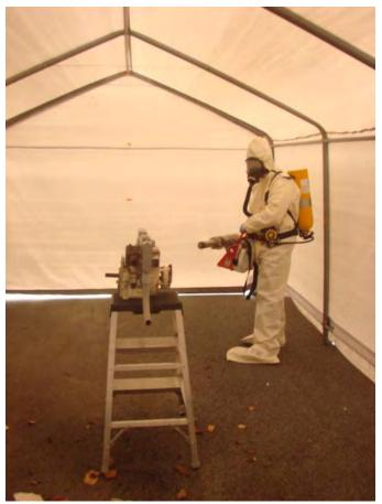
Directly applying the thermal fog to the engine.
