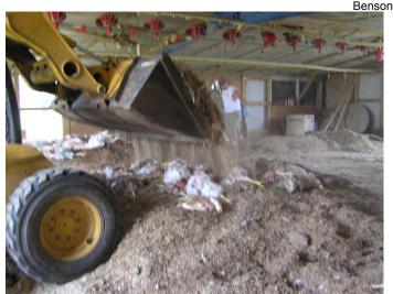
Skid steer loader constructing disposal windrow.
