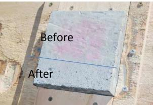
Coupon with dye before/after dry run
