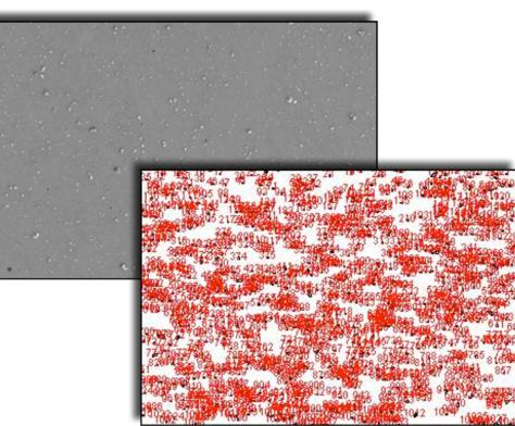
SEM/EDS images of contaminated surfaces CsCl deposition, particle density, and false color image for particle counting
