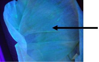
Very little simulant transfer observed on plastic from treated side of car
