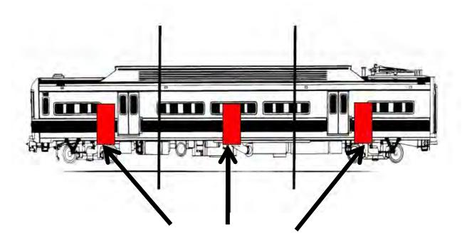
Contamination simulation powder applied to three areas of roughly the same dimension and location as the treated side of car
