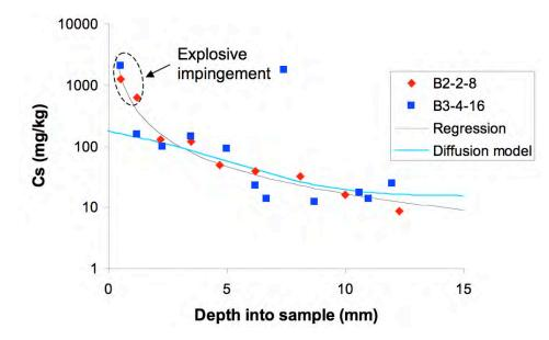
The migration into the concrete is believed to be due to diffusion, with Cs<sup>+</sup> carried in to the pores by the ambient relative humidity present between deposition and analysis (21-99 %RH over 32d).
