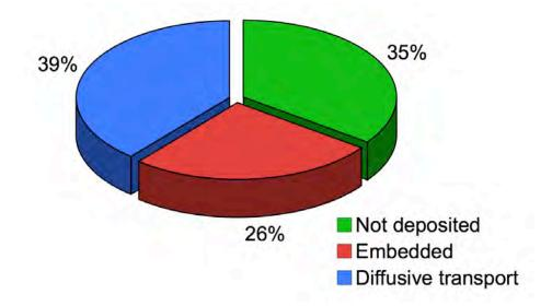
One third of the cesium was suspended, one quarter was explosively driven into the cement, the remainder underwent diffusion into the concrete, making decontamination problematic.
