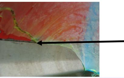
In area without pretreatment (zone 1) a substantial amount of simulant was observed in joint area after removal of stripcoat
