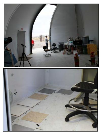
The aerosol chamber was chosen because of available instrumentation and ability to disperse a well mixed spore cloud (~4 log (10)) Surface Area~ 35.7 m<sup>2</sup> Volume~ 14.5 m<sup>3</sup>
