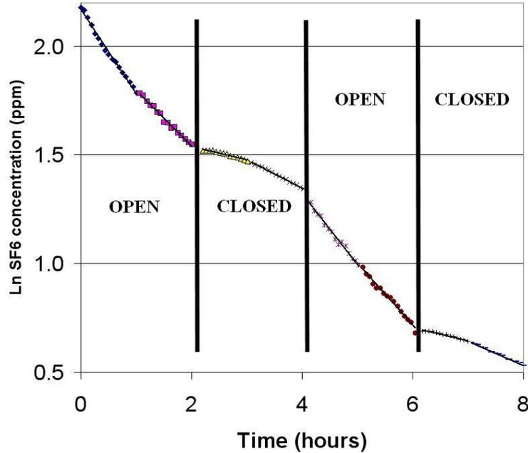
Figure 2: Example SF6 concentration data for a door open test, here opened once per minute, following tracer gas injection and mixing period.
