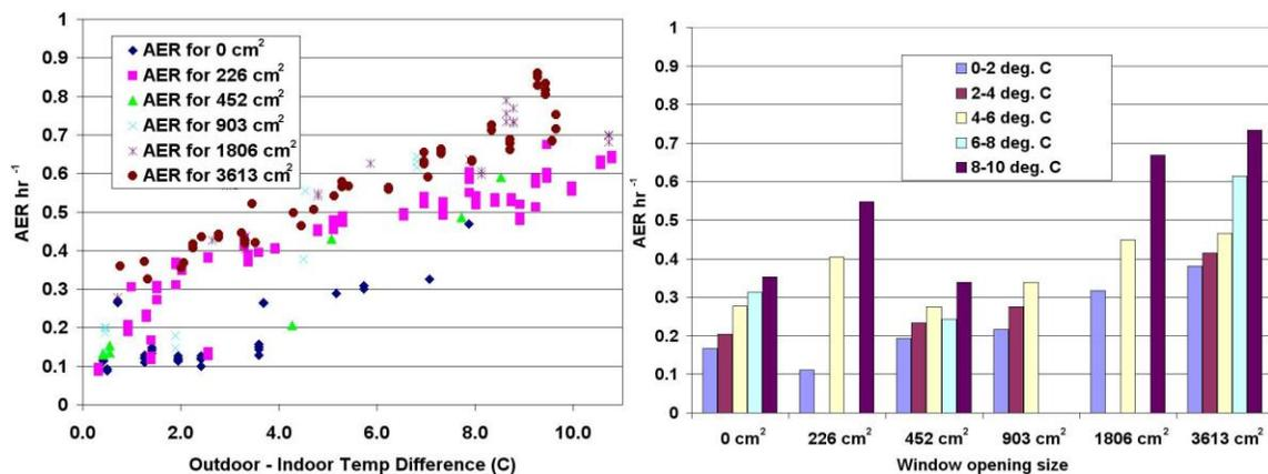
**Figure 4:** (Left) AER in each RTH room plotted against indoor to outdoor temperature difference for multiple window OAs. (Right) Average AER for the master bedroom plotted against window OA for multiple indoor to outdoor temperature differences.
