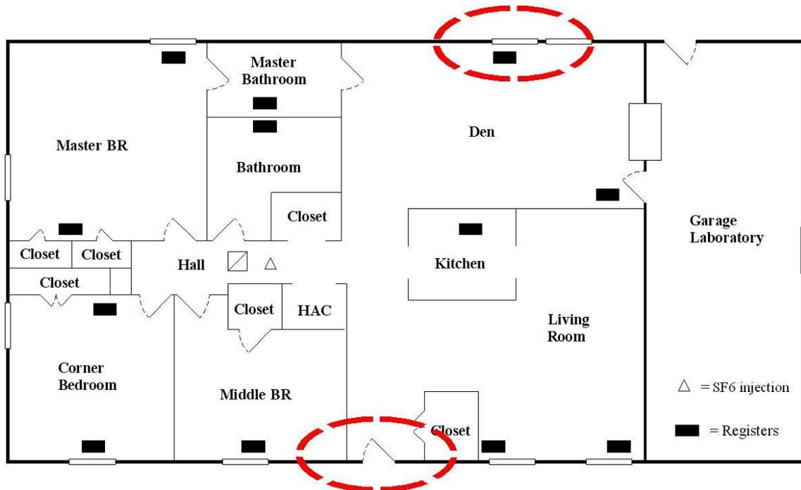
Figure 1: Layout of the single floor EPA research test house, located in Cary, NC, with circled locations of open door (bottom) and den window (top).
