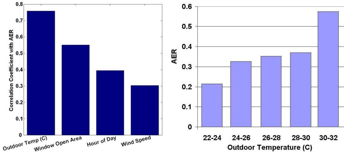
**Figure 3:** Correlation of measured parameters with AER for all outdoor temperatures and window OAs (left), for all outdoor temperatures over the HAC setpoint, including all window openings. On the right, AER (h<sup>-1</sup>) values for specific outdoor temperature ranges including all window OA.
