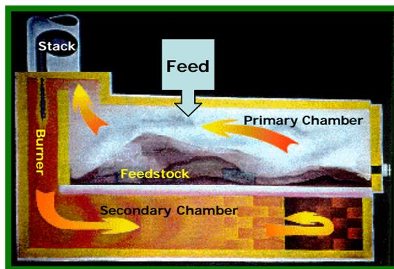
Figure 1. Gasifier Concept Schematic (Courtesy BGP, Inc.)
