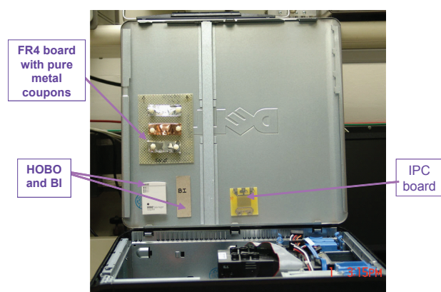
Figure 1-3. Location of HOBO®, Metal Coupons, IPC Board, and BI within the Computers (left side panel shown from a top-down view with respect to the computer).
