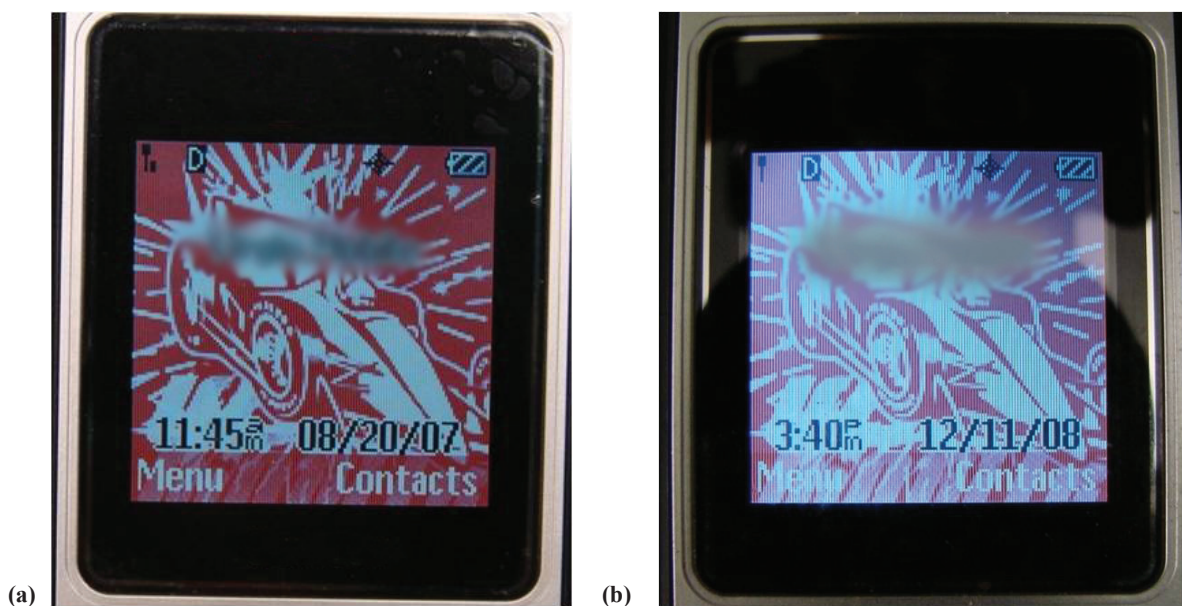
Figure 4-20. Cell phone screen (a) before and (b) at 12 months post-exposure to high RH fumigation (R06).
