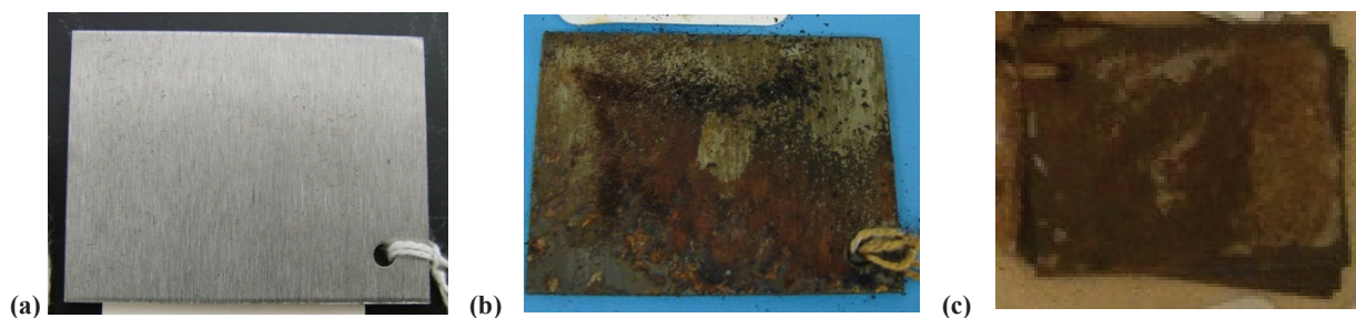
Figure 4-10. 410 Stainless steel coupons (a) before, (b) immediately after, and (c) at 12 months post-exposure to high RH fumigation (R06).
