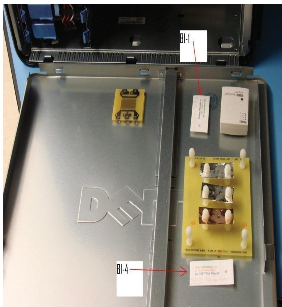
Figure 6-1. Location of two of the five BIs inside the computer side cover.
