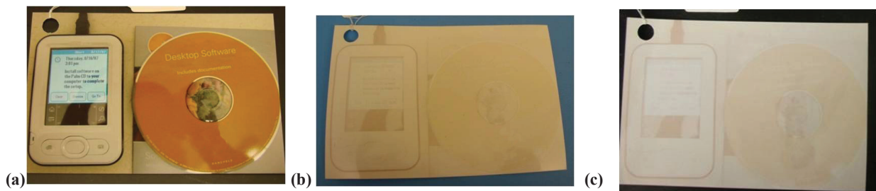
Figure 4-17. Photographs (a) before, (b) immediately after, and (c) 12 months post-exposure to high RH fumigation (R06).
