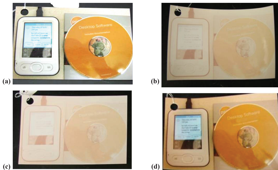
Figure 4-7. Photograph (a) before, (b) immediately after, and (c) at 12 months post-exposure to standard fumigation (R01), and (d) 12 months post-exposure to low concentration fumigation (R03).
