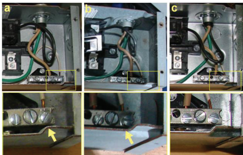
Figure 4-3. Corrosion on Cu service box at 12 months post-exposure to (a) low concentration fumigation (R03), (b) standard fumigation (R01), and (c) low RH fumigation (R04); lower pictures show a zoomed in area designated by the yellow boxes (arrows point out corrosion on edges of services).
