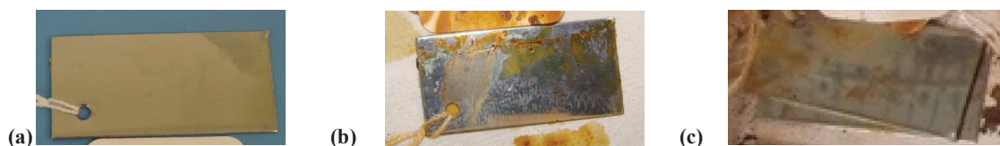
Figure 4-11. 430 Stainless steel coupons (a) before, (b) immediately after, and (c) at 12 months post-exposure to high RH fumigation (R07.)
