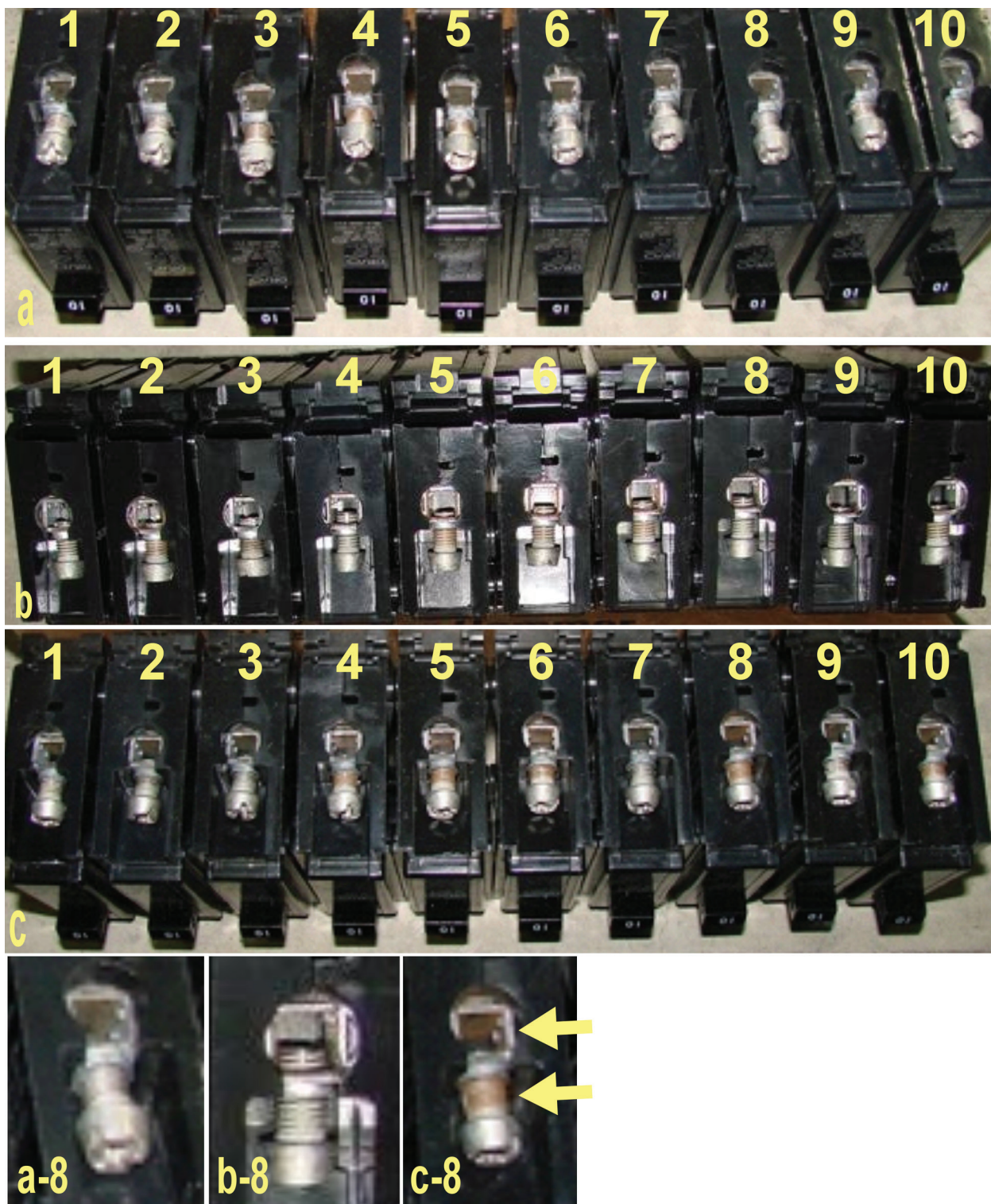
Figure 4-1. Corrosion on breaker screws at 12 months post exposure to (a) ambient conditions only (R05), (b) low RH fumigation (R04), and (c) high RH fumigation (R02); breakers are numbered 1-10 and a close-up of the screws for breaker 8 is shown. The arrows point to areas of corrosion evident on the screw on breaker 8 after exposure to high RH fumigation (labeled c-8 in the figure).
