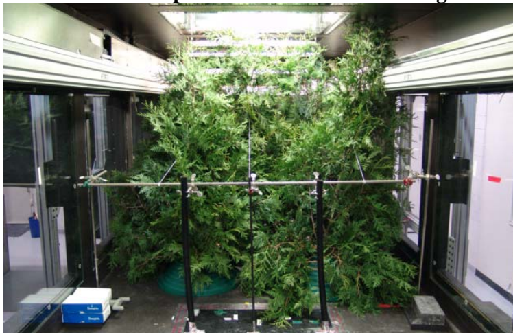
Figure 2. Wind tunnel experiment with needle leaf vegetative barrier
