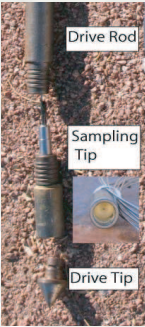
Figure 3: Photo of Micro-purge Vapor Probe Construction
