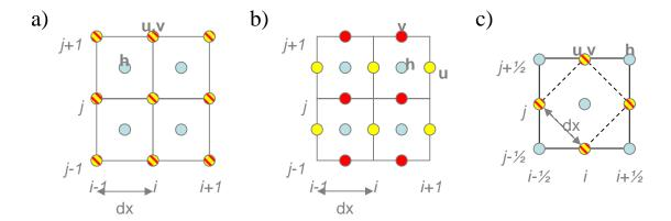
Figure 2. Graphical illustration of grid cells in an X-Y plane and the placement of the scalars ("h", shown in light blue) and the u- and v-components of the wind ("u" and "v", shown in yellow and red, respectively) on the (a) Arakawa B, (b) Arakawa C and (c) Arakawa E grids (based on Arakawa and Lamb, 1977).
