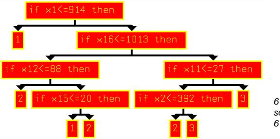
X1 = solar radiation (W/m<sup>2</sup>) X16 = air pressure (mbar) X12 = relative humidity (%) X11 = air temperature (C) X15 = dewpoint (C) X2 = solar radiation at fire department met station (W/m<sup>2</sup>)
