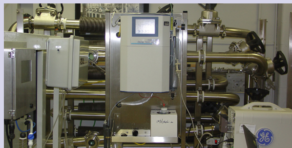
Participating technologies shown connected to EPA's portable pipe loop.
