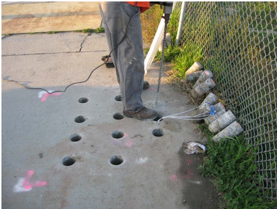
Photograph 2: Concrete core holes at location ST-2
