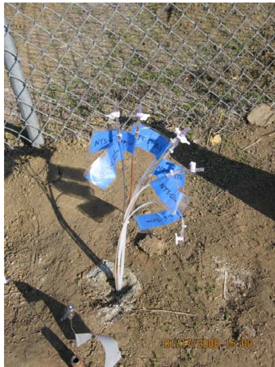
Photograph 9: EPA installing micro-purge soil gas probes.
