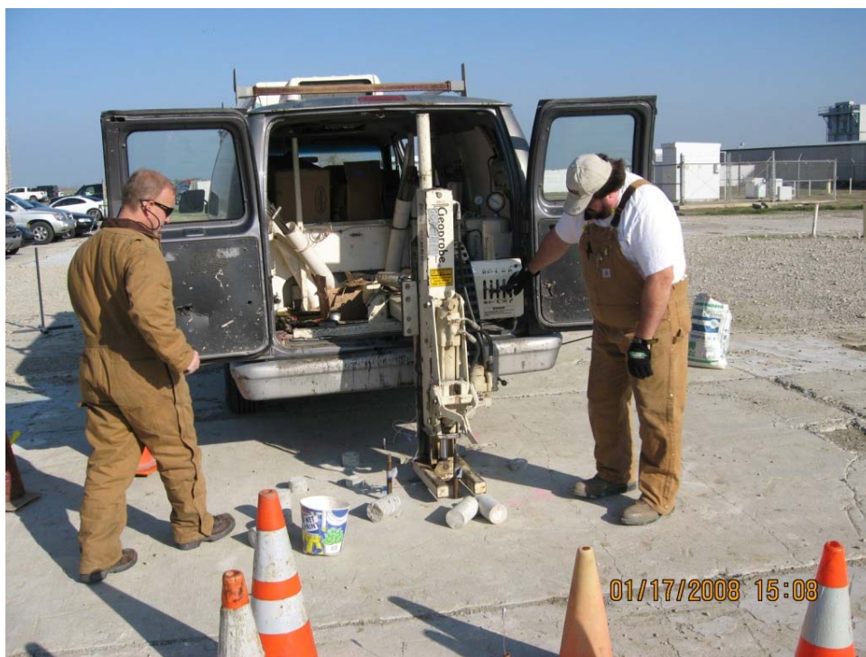
Photograph 8: EPA installing micro-purge soil gas probes.
