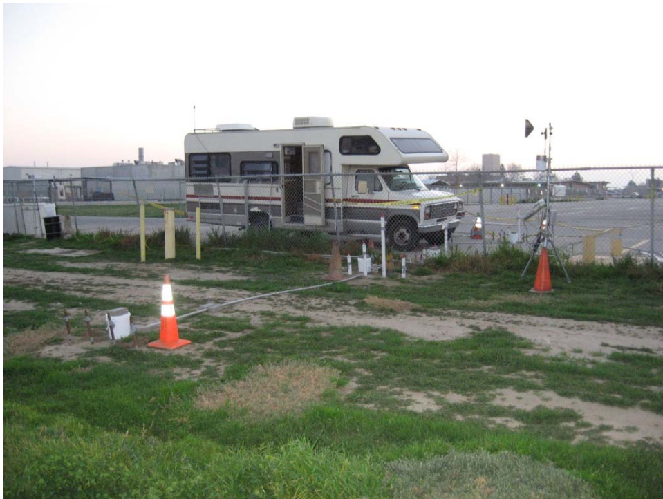
Photograph 18: Auto-sampler RV. Conduit running from probe locations to RV visible in middle ground.
