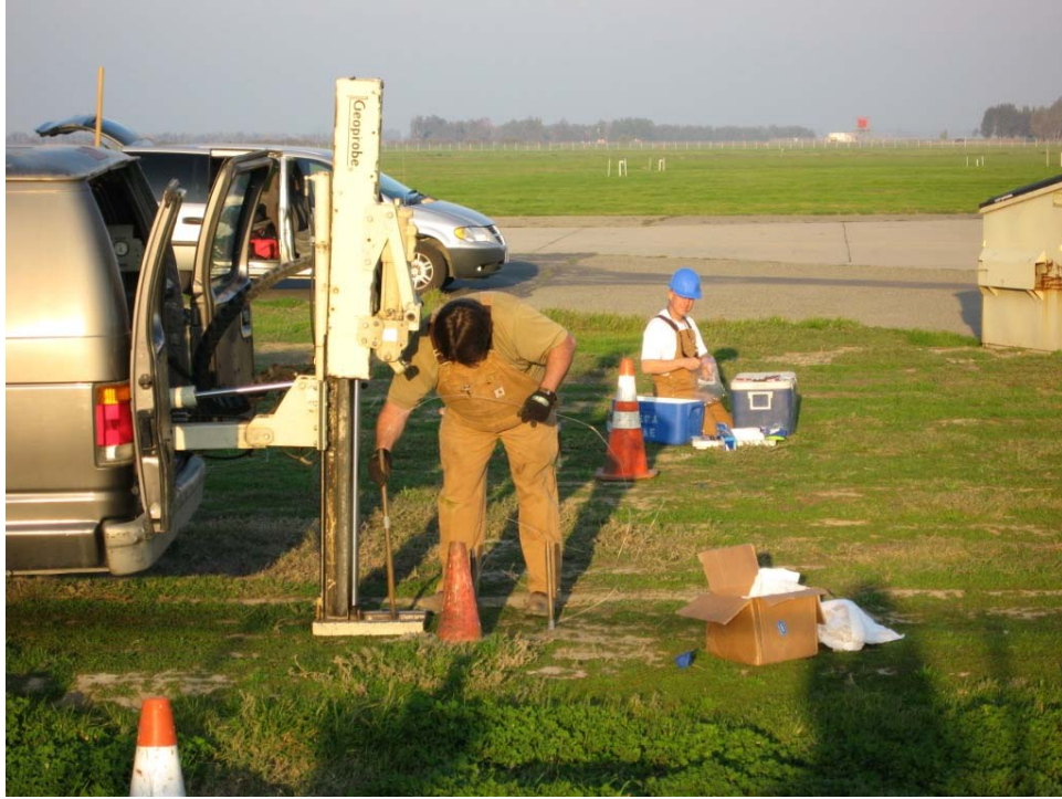
Photograph 9: EPA installing micro-purge soil gas probes.
