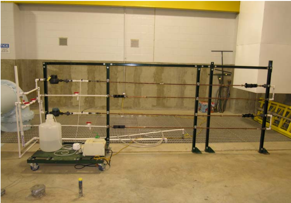
FIGURE 1. Photograph of copper pitting corrosion evaluation pipe loop apparatus.
