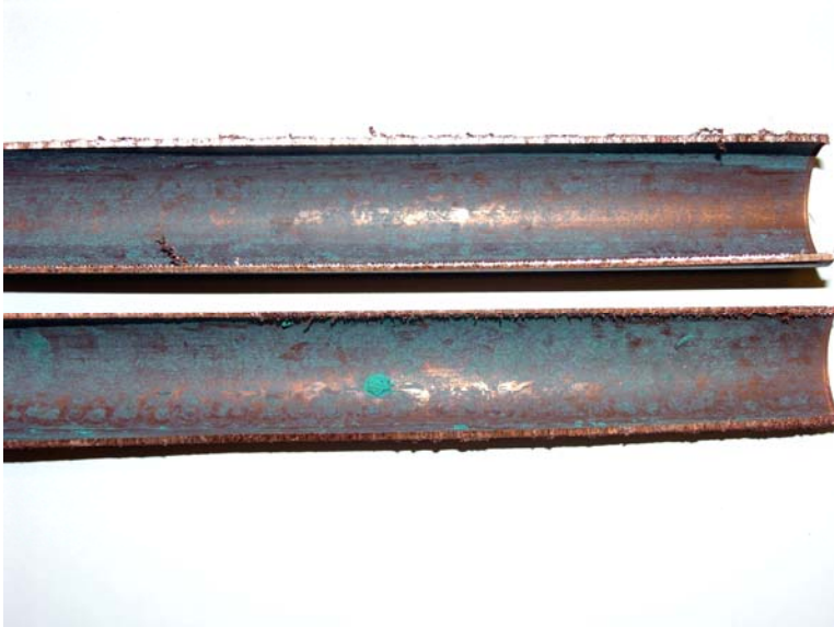
FIGURE 3. Interior surface of copper pipes removed after 101 days:
