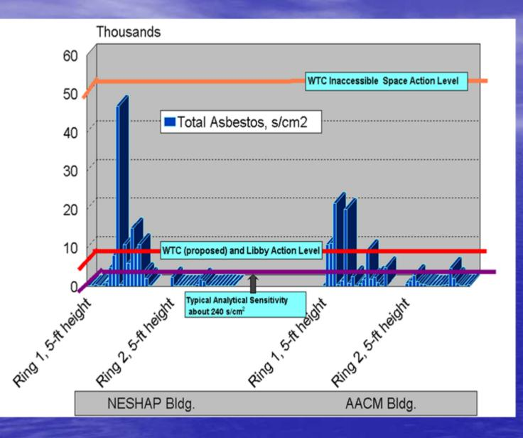
AACM1 Dust Asbestos Loading, s/cm<sup>2</sup>
