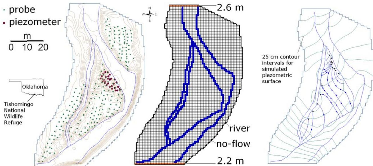
Figure 1. Left: Map of contoured elevations (10 cm intervals), probe locations, and piezometer locations, Middle: MODFLOW discretization, Right: Results displayed as flow net (arrows show 24-hr time intervals).
