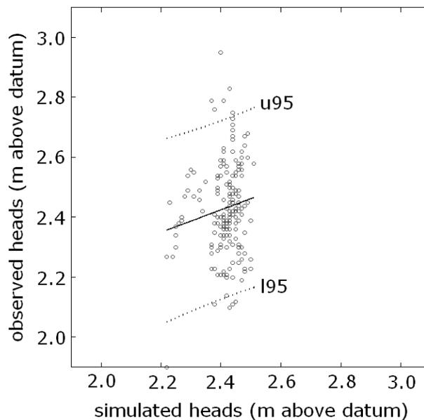
Figure 2. Plot of simulated versus probe-observed heads. Linear regression:  $y = 1.53 + 0.37x$ ,  $r^2 = 0.02$ ,  $p = 0.05$ . Upper and lower 95% confidence limits shown.
