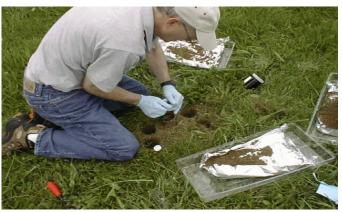
Picture 2. Sampling Using the Bulb Planter Method
