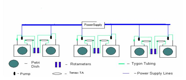
The experimental setup allows for easily introducing the sorbent tubes into the sample loop, without the need to open the growth chambers. A miniature pump draws the headspace from the chambers into the sorbent tube. The sample loop continues to a rotameter, where airflow is measured, and is then transferred back into the growth chambers, thus providing a completely enclosed sample system
