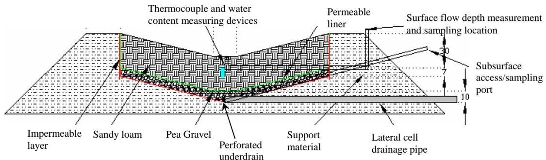
**Figure 2.** Schematic of swale cross-section.
