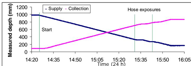
Figure 4. Measured depths in supply and collection tanks during a trial run.
