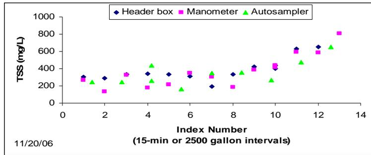
Figure 6. TSS concentrations measured in samples collected at 15-minute interval from the header box and manometers and samples collected at 9500-l (2500 g) intervals by the autosampler.
