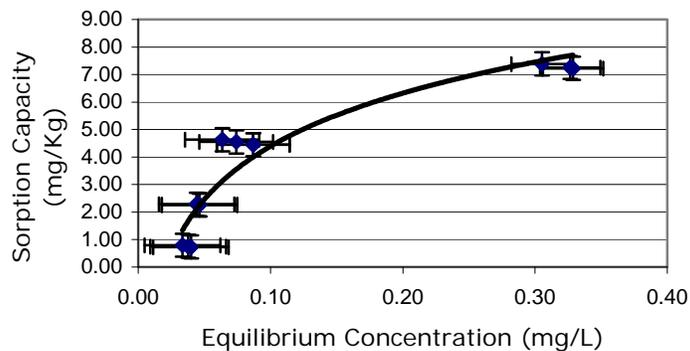
Figure 5. Copper isotherm data for the NJ infield mixture.
