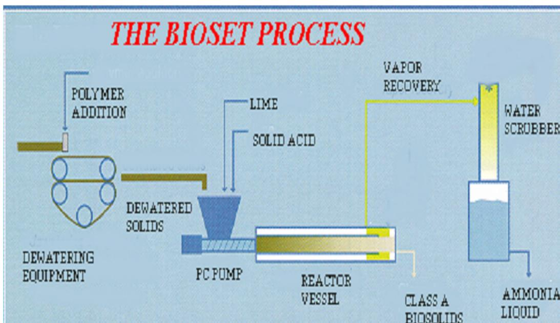
Significant heat is produced as calcium oxide, quicklime, is added at a level of 40-50% dry weight to dewatered sludge. The calcium hydroxide, produced from this reaction, reacts with the sulfamic acid to produce even more heat. Since the calcium oxide to sulfamic acid ratio is approximately 100:1, the pH of
