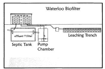
Generalized design of the Waterloo Biofilter System.
