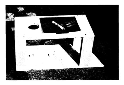
A bilge compartment port size-test device was constructed as shown in the plans in Figure 2. The purpose of this device was to ensure that the product could be retrieved from boat bilge compartments with 3.5" openings after becoming saturated with hydrocarbons.
