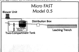
Generalized schematic of the MicroFAST Model 0.5.
