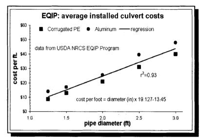
**Figure 7.** Simplified cost assumptions for culvert installation based on USDA-NRCS model for farm apllications (i.e. not typically paved roads.
