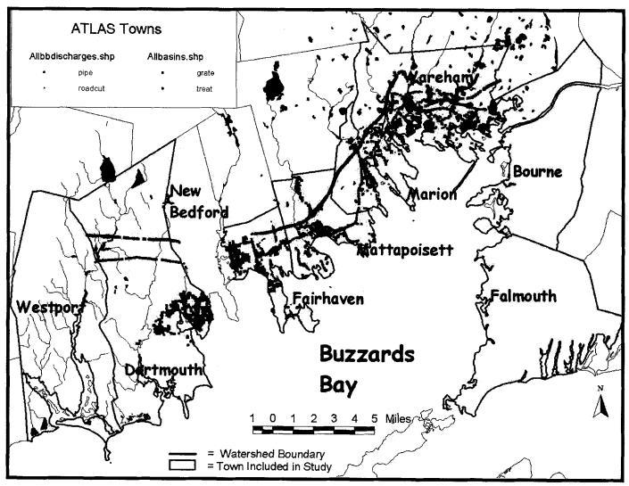
Figure 8. Map pf all storm drains, road cuts, and catch basins in Buzzards Bay watershed communities. This map is too large a scale to show individual discharge pipes and basins and is provided here to give the reader a sense of the scope of the stormwater discharge inventory.
