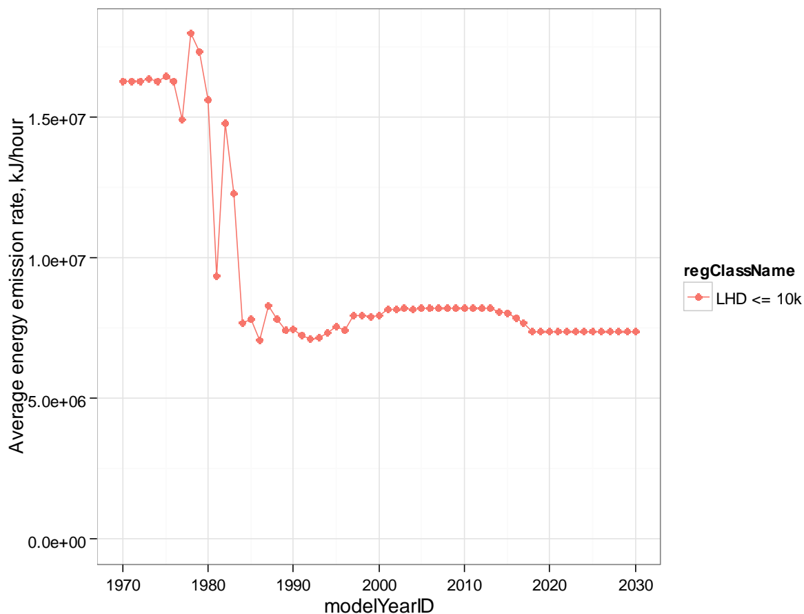
Figure 3-15. Average Energy Consumption Rates for LHD<=10K gasoline vehicles across all running operating modes
