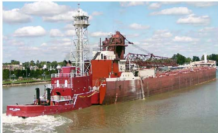
Figure 7-14 Example of a Former Freighter Turned Barge: The Lewis J. Kuber Pushed by the Olive Moore
