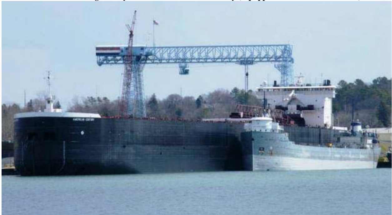
Figure 7-11 The St. Mary's Challenger (Built with a Forward Pilothouse and Pictured on the Right) Spends the Winter in Sturgeon Bay next to the American Century (Equipped with a Rear Pilothouse)
