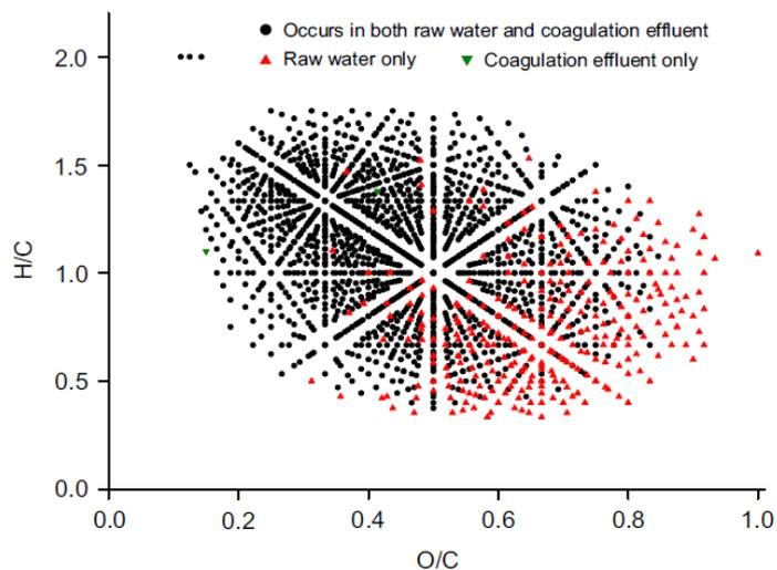
Fig. 2 – The van Krevelen diagram of the raw water DOM overlain with the coagulation effluent DOM.
