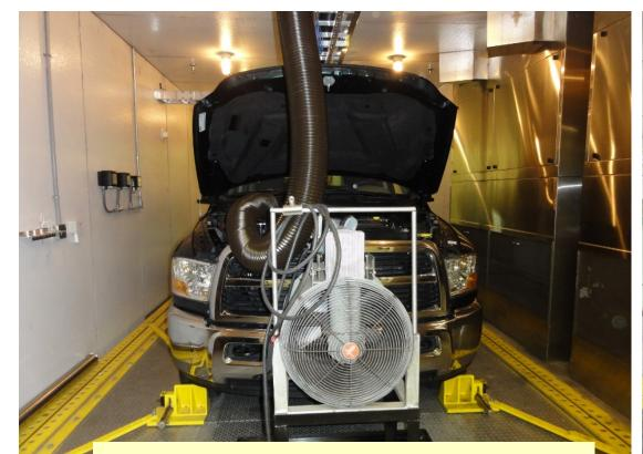
Light-duty Dynamometer: 48 in. roll Capacity: 12,000 lbs Temp: -30 to 43 °C Heavy-duty Dynamometer: 72 in. roll Capacity: 30,000 lbs Temp: 22 ° C
