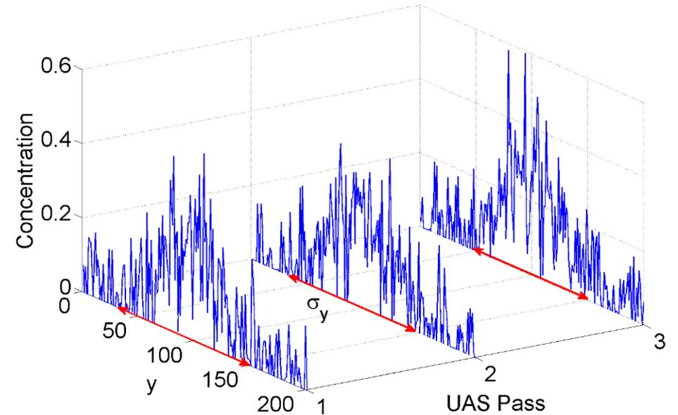
Mobile measurement of plume transects can help estimate plume dispersion and source strength
