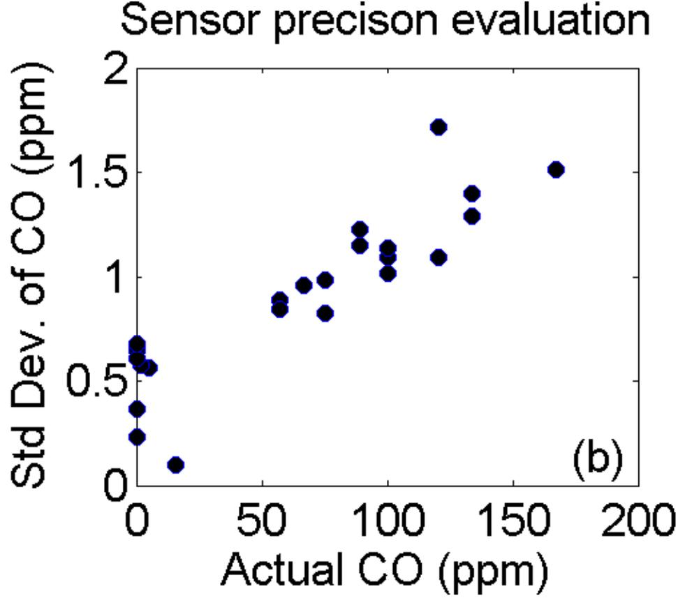
Sensor is accurate and precise at high concentrations relevant for this application
