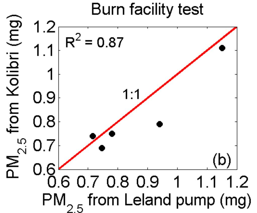
PM<sub>2.5</sub> unit maintains 10 L/min based on a pressure sensor and performed well when comparing against a standard pump
