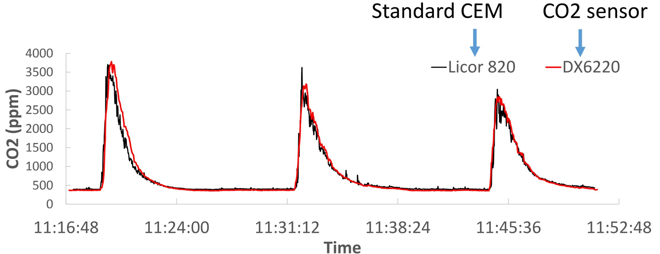
CO<sub>2</sub> sensor tracks reasonably well with the Licor 820 instrument at high concentrations relevant for this application
