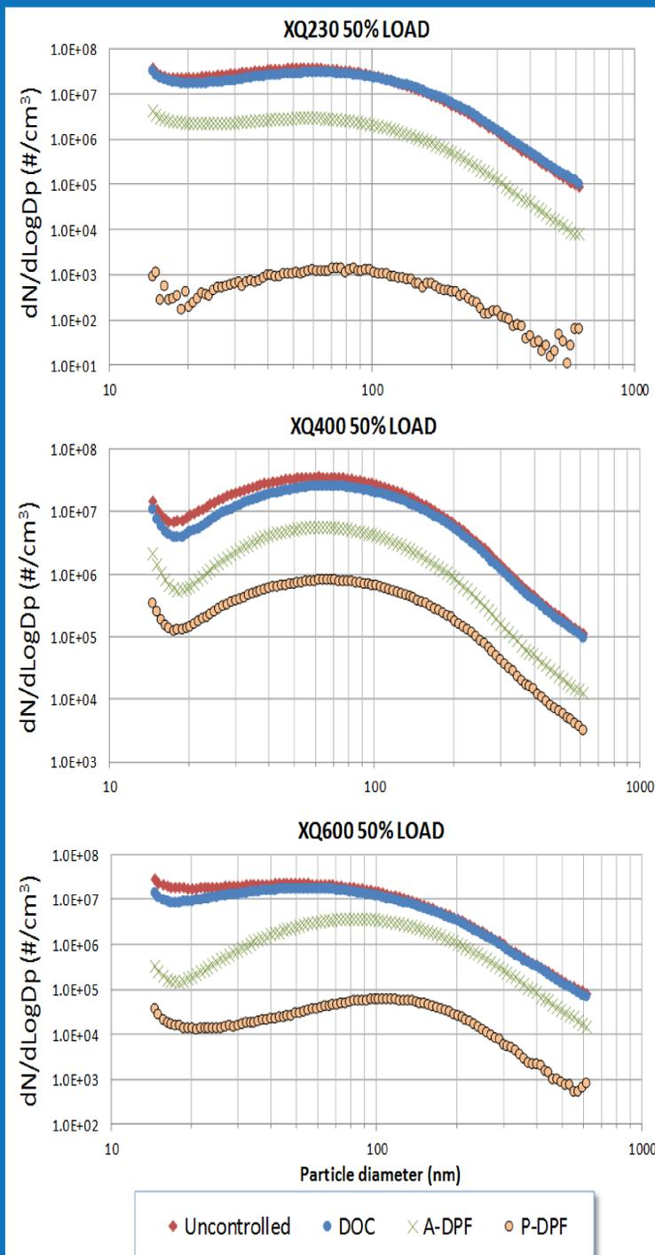
Figure 1: Particle size distribution at 50% load for (a) XQ230, (b) XQ400, and (c) XQ600 with and without aftermarket controls (similar trends occur for each genset at 90% load)
