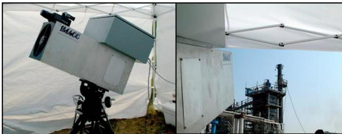
The instrument was deployed from the back of a field trailer, and was mounted on a mechanical positional scanner. At each measurement site, the trailer was oriented to provide a clear line of sight between the PFTIR and the emissions source detected during the pre-measurement OGI camera survey. Measurements were collected at  $0.5 \text{ cm}^{-1}$  spectral resolution, and the instrument field of view was approximately 14" in diameter. Each data point was averaged for 30 seconds,
