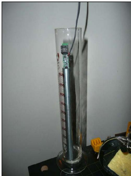
**Figure 3. Capacitance and Conductance (Complex Impedance) (C/C)**
