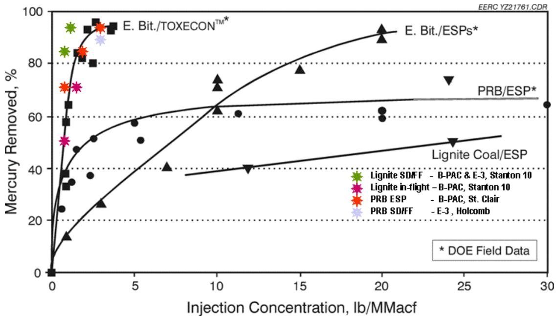
**Figure 14.** Results from DOE-sponsored 30-day full-scale testing at DTE St. Clair 80 MW boiler with CS-ESP, firing PRB and an 85:15 PRB:bituminous blend and using B-PAC.<sup>54</sup>
