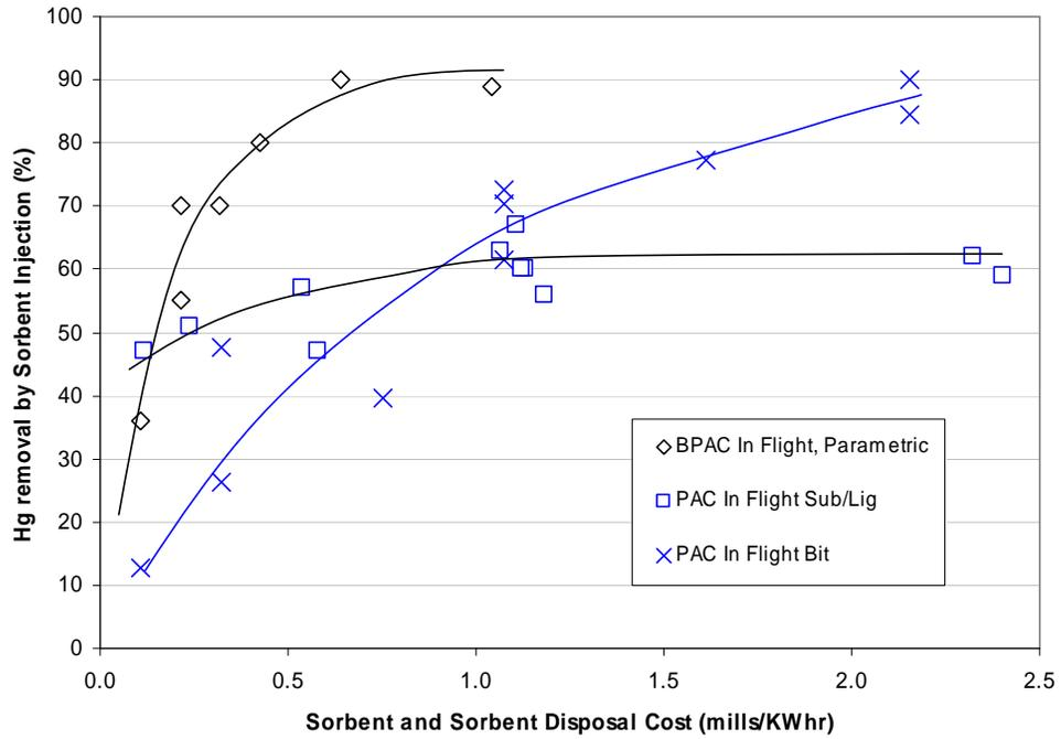
**Figure 20.** Estimated sorbent and disposal costs for sorbent injection upstream of an FF.
