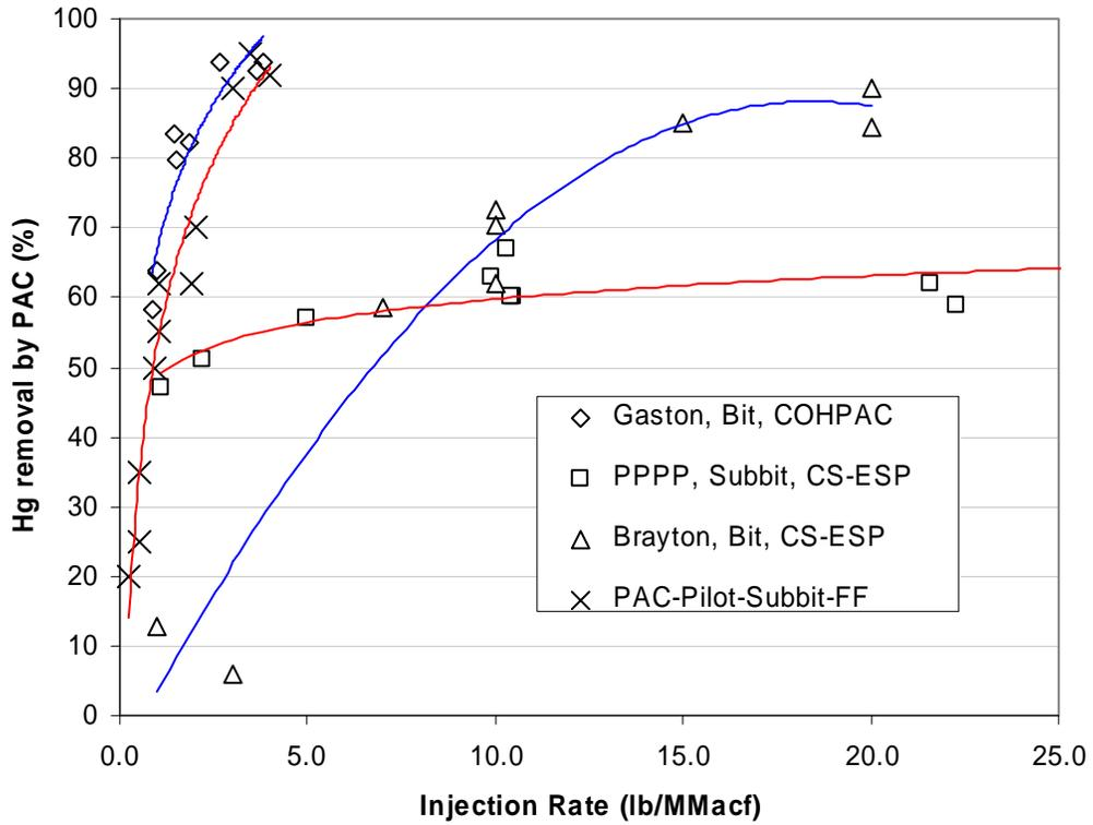
**Figure 9.** Results of relatively long-term PAC testing at Gaston <sup>52</sup>
