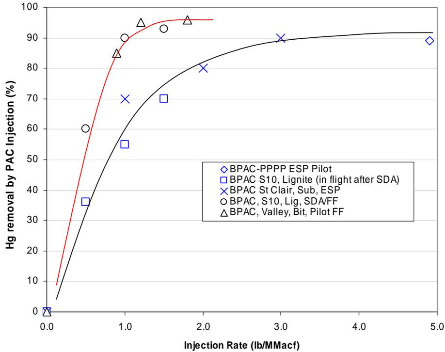
**Figure 13.** Performance of halogenated PACs versus that with standard PACs.<sup>53</sup>
