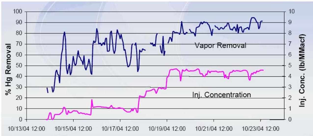
**Figure 16.** Results from DOE-sponsored 30-day full-scale testing at Holcomb 360 MW boiler with SD+FF, firing PRB blend and using Norit E-3.<sup>55</sup>
