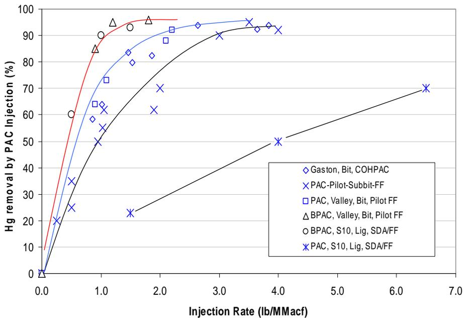
**Figure 12.** Performance of B-PAC in parametric tests are shown for in-flight and upstream of a fabric filter for various coal types.
