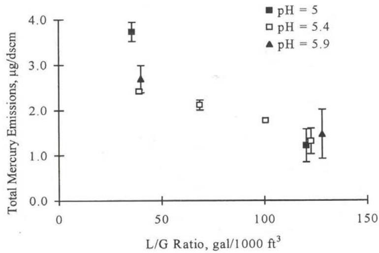
Figure 5. Mercury removal of various FGD systems
