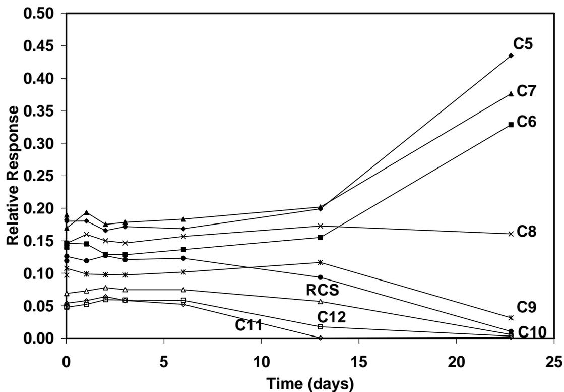
Fig. 5. Time-concentration profile of PFCA standards (1 ng/mL) in glass bottle at room temperature (about 23 °C; RCS is recovery check standard).
