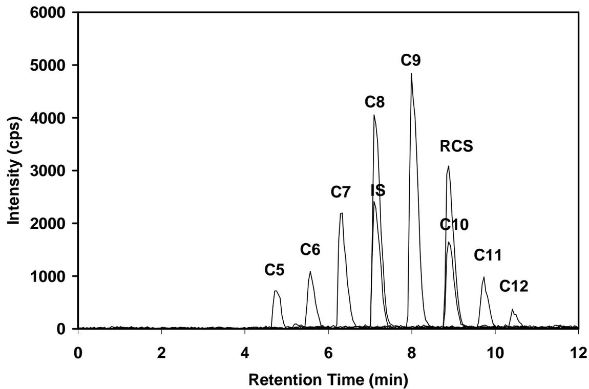
**Fig. 1. Chromatogram of a non-woven medical garment sample (IS is internal standard, RCS is recovery check standard).**
