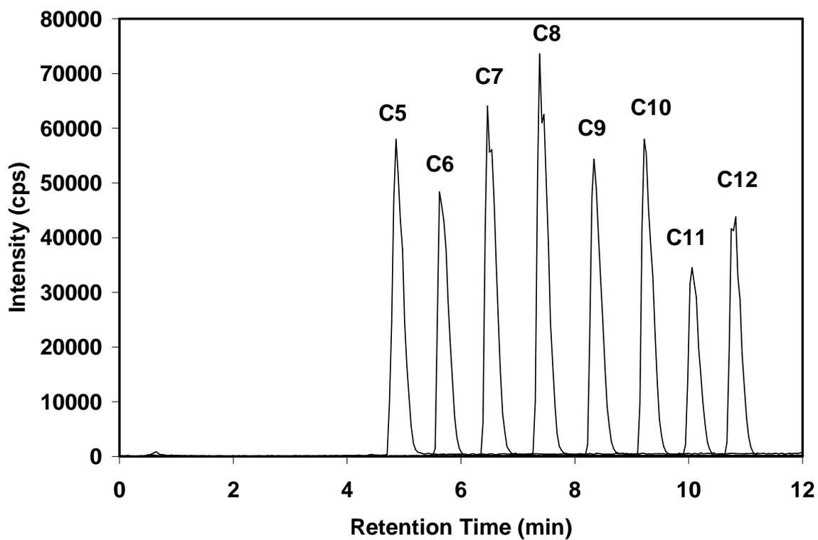
**Fig. 2b. The effect of solvent composition for preparing the injection solution on LC/MS/MS performance -- Case 2: 60% (v/v) methanol and 40% 2 mM NH<sub>4</sub>Ac aqueous solution (showing good sensitivity and peak resolution).**
