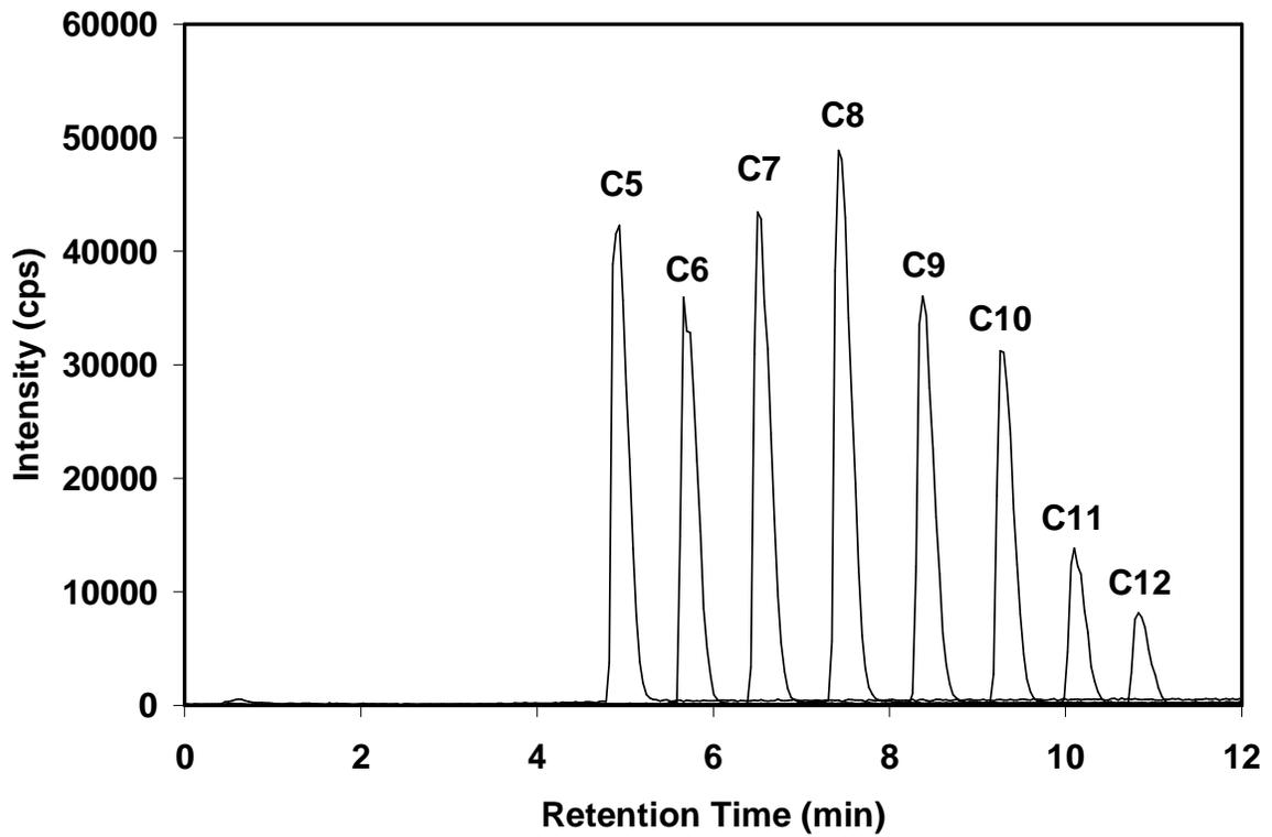
**Fig. 2c. The effect of solvent composition for preparing the injection solution on LC/MS/MS performance – Case 3: 10% (v/v) methanol and 90% 2 mM NH<sub>4</sub>Ac aqueous solution (showing good peak resolution but low sensitivity).**
