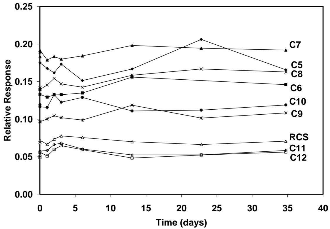
**Fig. 4. Time-concentration profile of PFCA standards (1 ng/mL) in polypropylene conical centrifuge tubes in refrigerator at about 4 °C (RCS is recovery check standard).**
