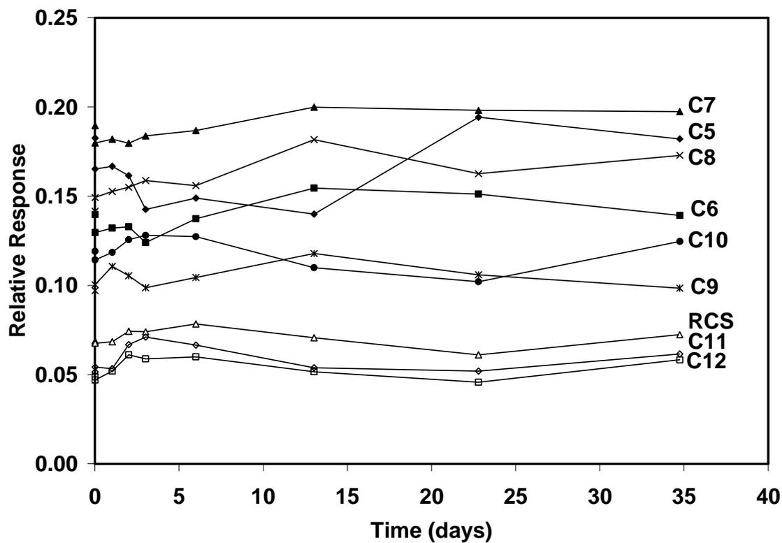
**Fig. 6. Time-concentration profile of PFCA standards (1 ng/mL) in polypropylene conical centrifuge tubes at room temperature (about 23 °C; RCS is recovery check standard).**
