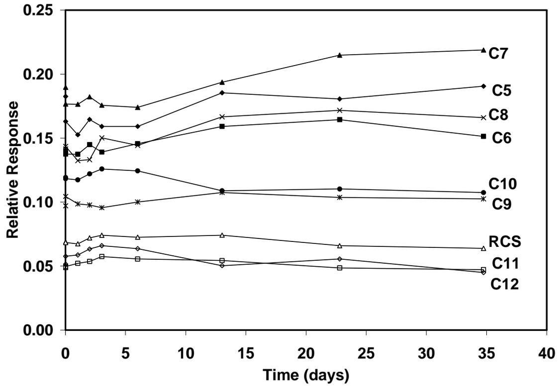
**Fig. 3. Time-concentration profile of PFCA standards (1 ng/mL) in glass bottle in refrigerator at about 4 °C (RCS is recovery check standard).**
