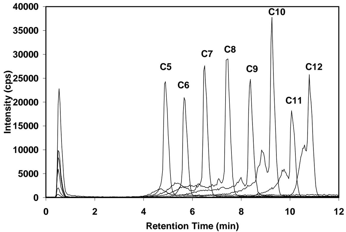
**Fig. 2a. The effect of solvent composition for preparing the injection solution on LC/MS/MS performance – Case 1: 100% methanol (showing peak doubling).**
