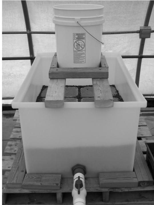
**Figure 2. Bench-scale pervious pavement system demonstrating stormwater delivery method.**
