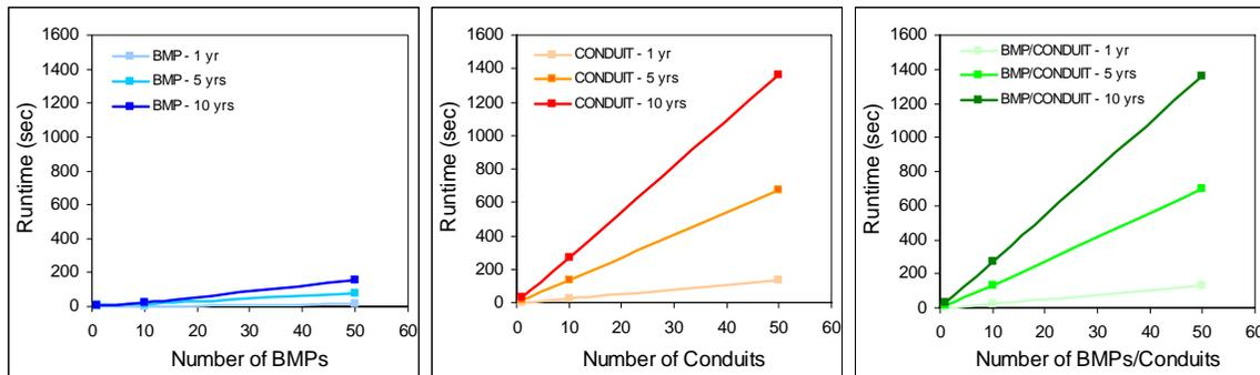
**Figure 3 – Runtime comparison of various number of simulation units (BMP, conduit, or BMP/conduit combination) and of various simulation periods.**
