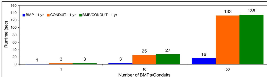
**Figure 4 – Runtime comparison of various simulation units (BMP, conduit, or BMP/conduit combination) for a 1-y simulation period.**
