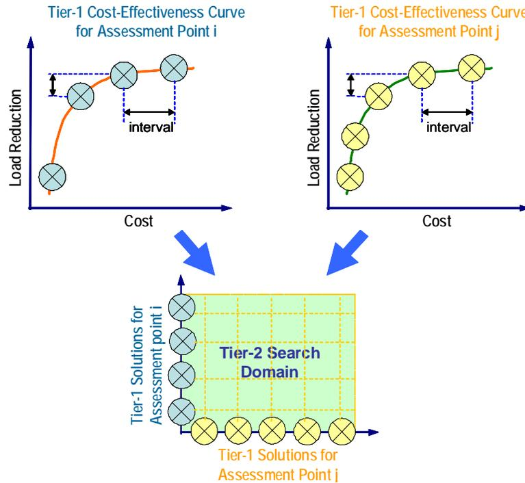
**Figure 6 - Construction of the tier-2 search domain using tier-1 results.**
