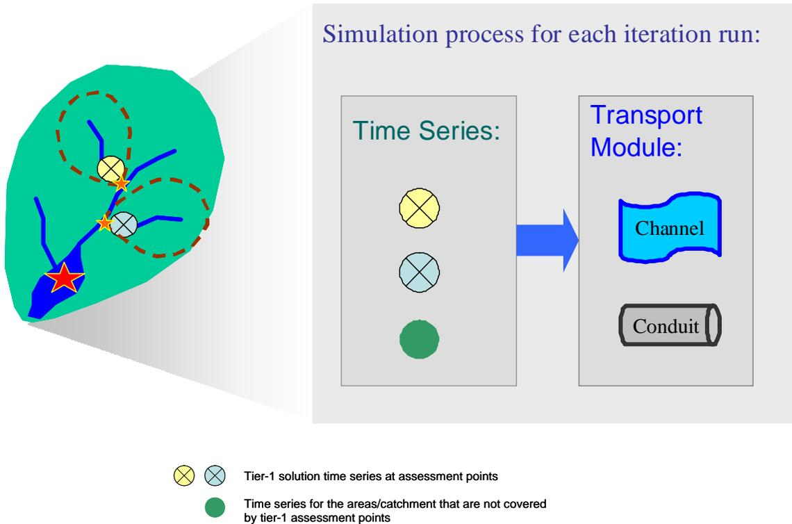
**Figure 7 - Simulation process for each iteration run.**
