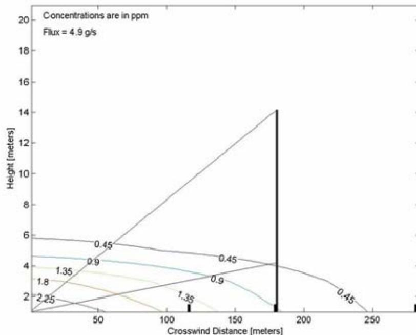
**Figure 16. Reconstructed methane plume map from the VRPM survey of the Colorado Springs, CO site (concentrations shown in ppmv). The location of the vertical structure is shown by the solid black vertical line. The scanning ORS instrument is located in the bottom left-hand corner of the figure**
