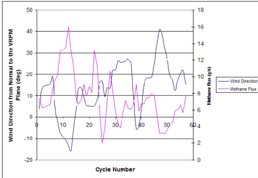
**Figure B-6. Time series of wind direction and methane flux values from the May 4 VRPM survey of Survey Area #2 using the Boreal OP-TDLAS**
