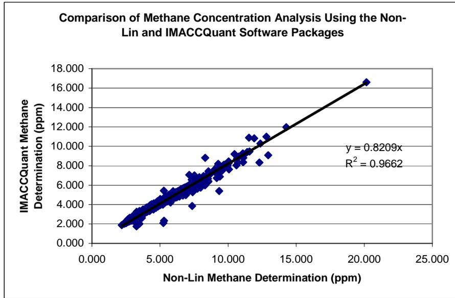
**Figure 31.** Comparison of methane concentration analysis using the Non-Lin and IMACCQuant software packages
