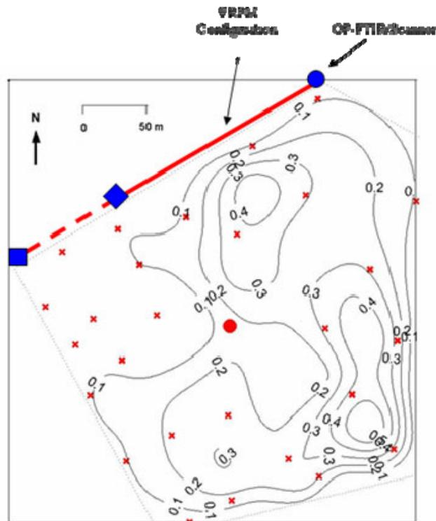
**Figure 15.** Surface methane concentration contours (in ppmv) overlaid on the map of the Colorado Springs, CO site. The figure shows the location of the VRPM configuration at the site
