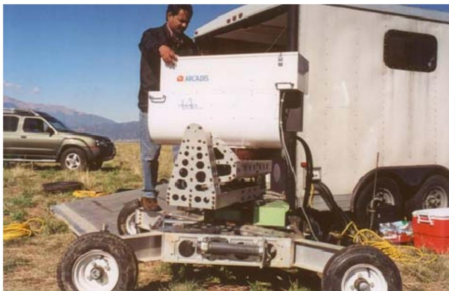
Figure 6. Unisearch Associates OP-FTIR instrument and scanner
