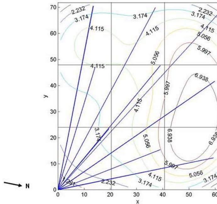
**Figure B-2. Average Methane Surface Concentration Contour Map from the May 3 HRPM Survey of Area #2 (concentrations shown are in ppm above background)**
