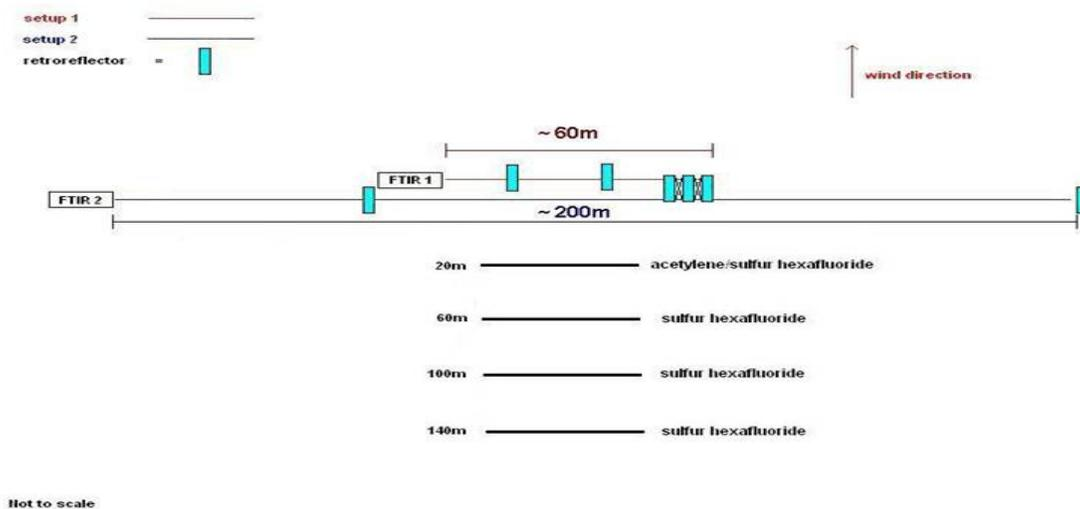
**Figure 24. Schematic of the experimental configuration used for the VRPM validation study**
