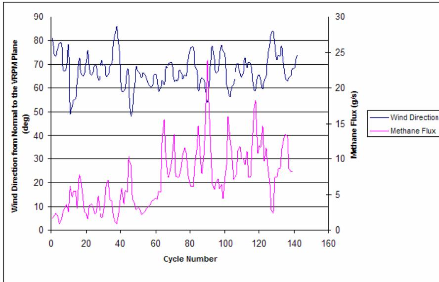
**Figure B-7. Time series of wind direction and methane flux values from the May 5 VRPM survey of Survey Area #2 using the Boreal OP-TDLAS**
