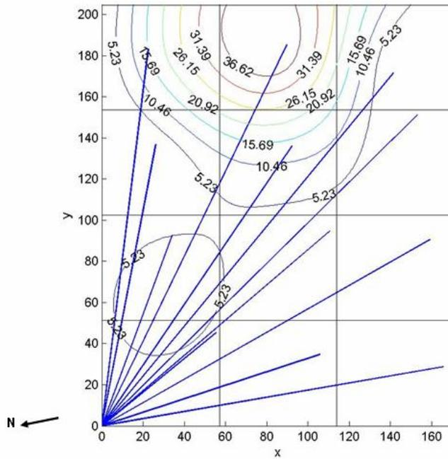
**Figure B-9. Average Methane Surface Concentration Contour Map from the May 3 HRPM Survey of Area #2 (concentrations shown are in ppm above background)**
