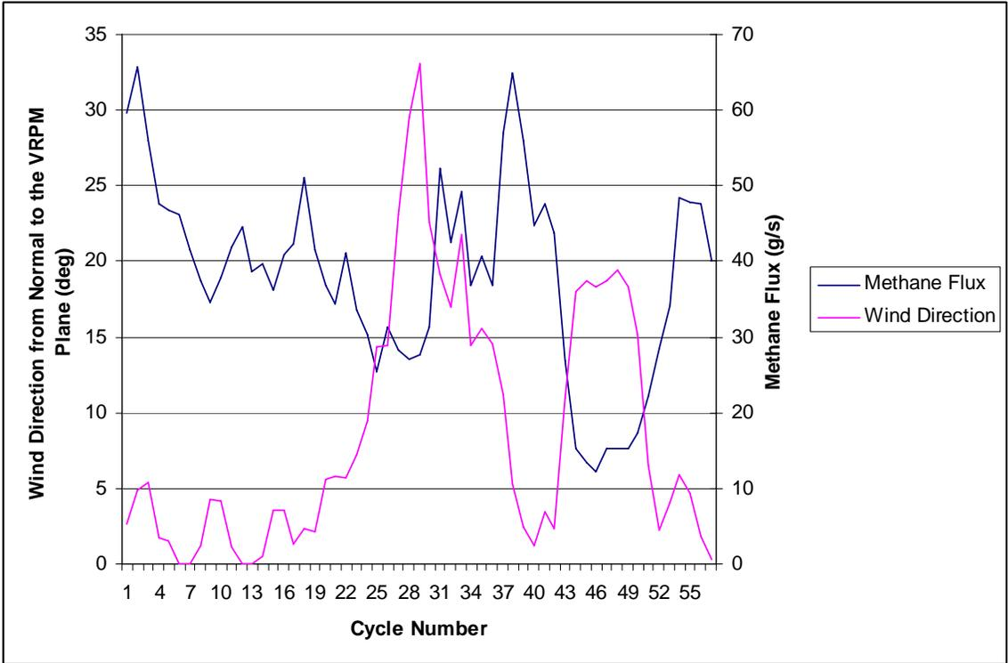
Figure C-2. Time series of wind direction and methane flux values from the June 19 VRPM survey.
