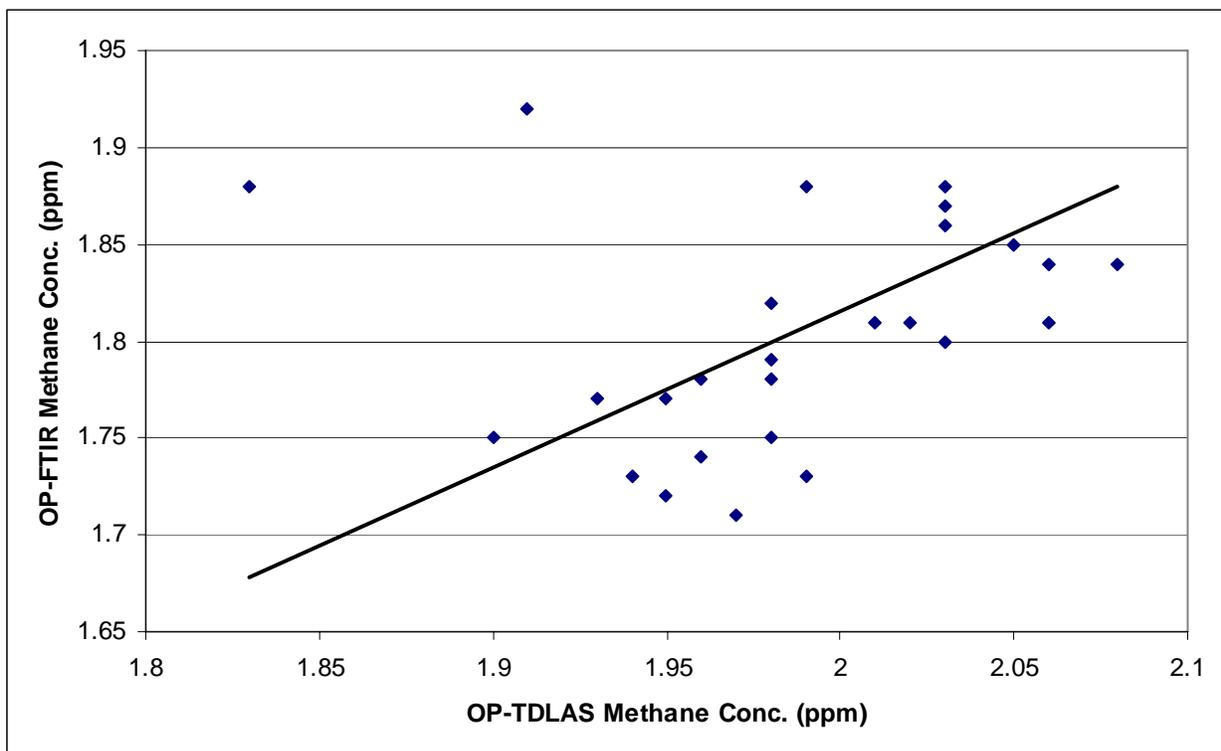
**Figure 11. Comparison of methane concentrations measured along similar beam paths during the Fort Collins measurement campaign with the OP-FTIR and OP-TDLAS instruments**
