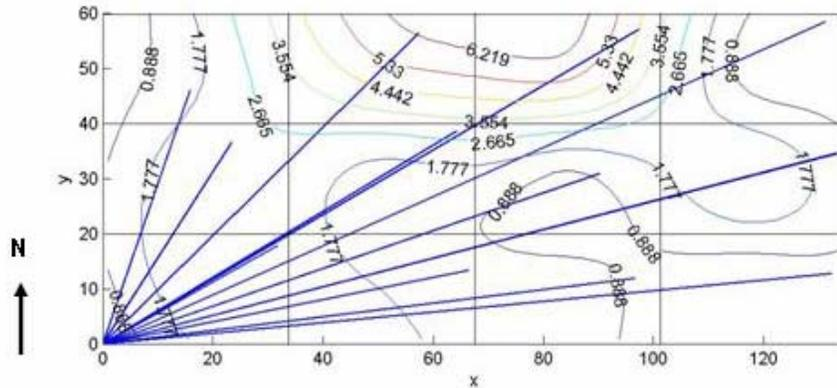
**Figure B-1. Average Methane Surface Concentration Contour Map from the May 2, 2006 HRPM Survey of Area #1 (concentrations shown are in ppm above background)**
