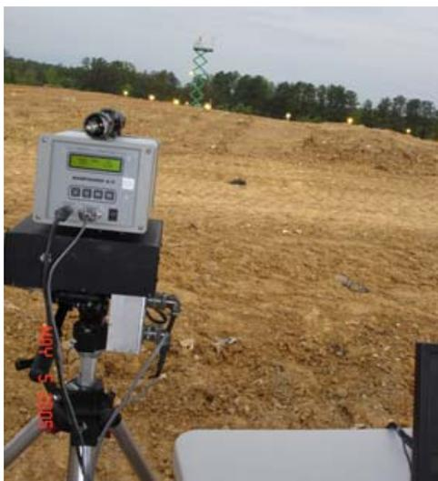
Figure 9. Boreal OP-TDLAS system and scanner
