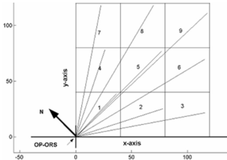
Figure 1. Example HRPM configuration showing the location of the ORS instrument, and the beam paths used for the survey
