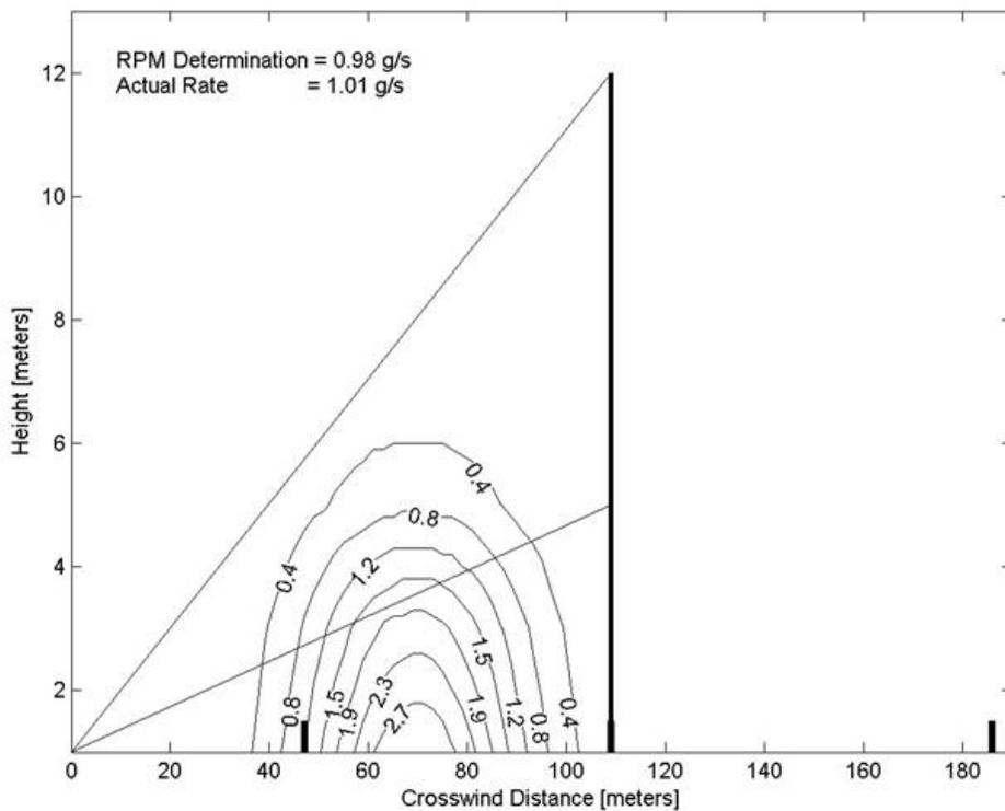
**Figure 30.** Reconstructed ethylene plume from the VRPM validation study conducted during the Somersworth, NH field campaign (concentrations shown in ppmv). The location of the vertical structure is shown by the solid black vertical line. The scanning ORS instrument is located in the bottom left-hand corner of the figure
