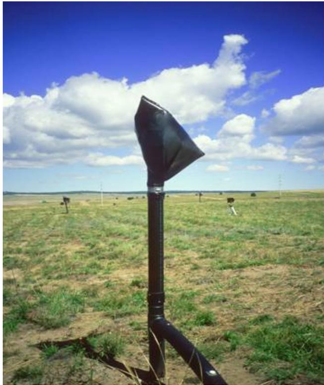
**Figure 17. Passive vents sealed with plastic at the Colorado Springs site**
