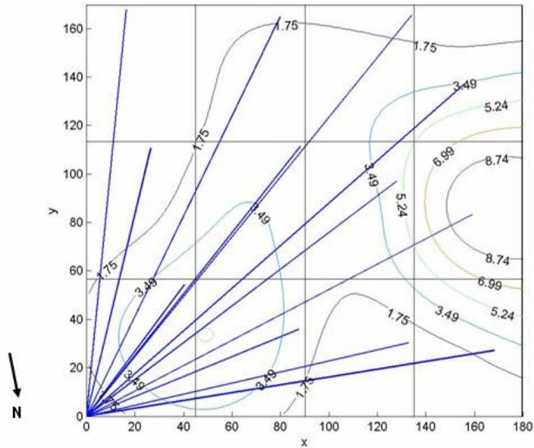
**Figure B-8. Average Methane Surface Concentration Contour Map from the May 2 HRPM Survey of Area #1 (concentrations shown are in ppm above background)**
