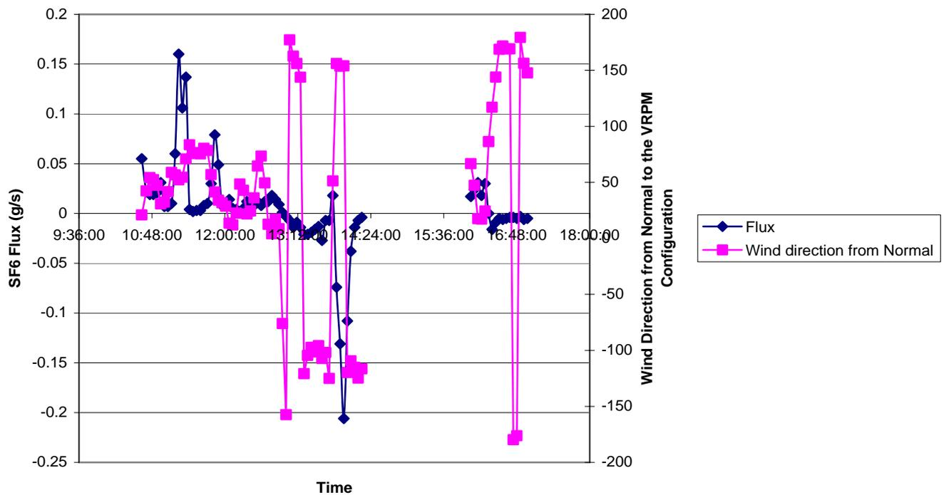
Figure 25. Time series of wind direction and calculated sulfur hexafluoride fluxes from the 20 meter release (as analyzed along the 200 meter VRPM configuration)
