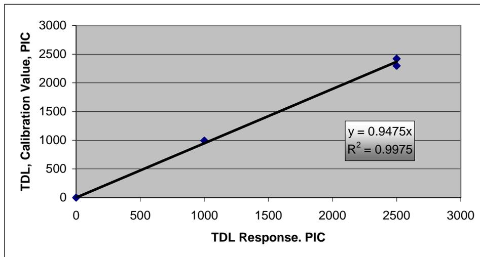
**Figure 29. Plot of the Unisearch OP-TDLAS instrument calibration response**
