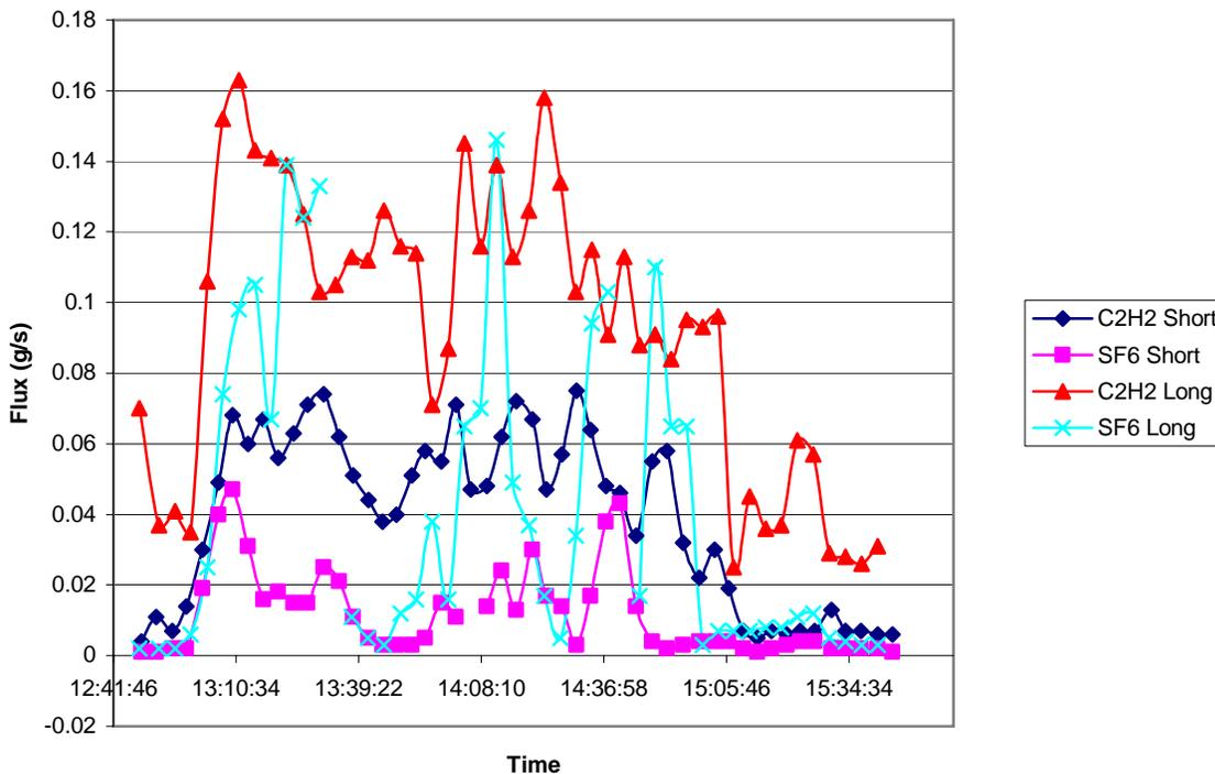
**Figure 28. Time series of acetylene and sulfur hexafluoride flux values from the 140 meter release survey**
