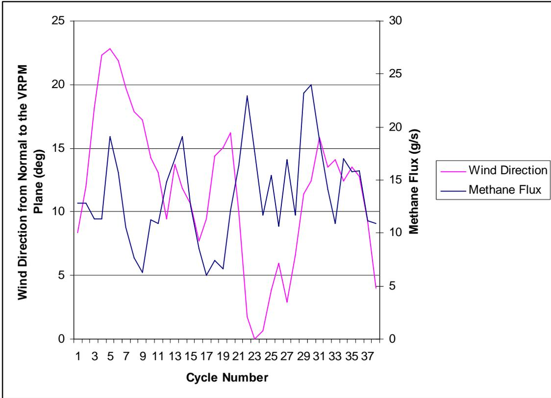
Figure C-6. Time series of wind direction and methane flux values from the July 7 VRPM survey.
