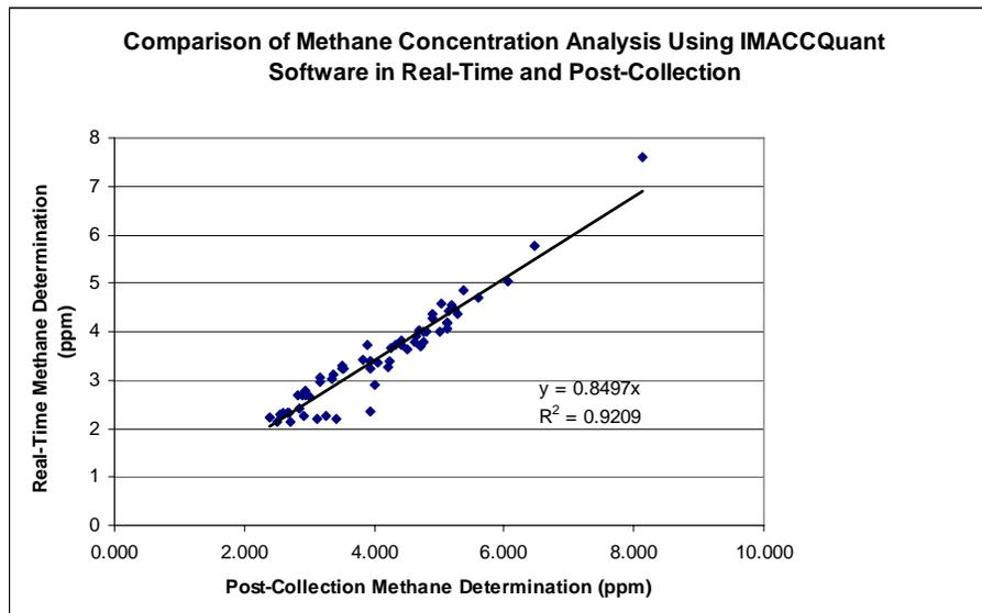
**Figure 32.** Comparison of real-time and post-collection methane concentration analysis using the IMACCQuant software package
