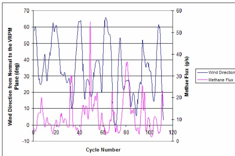
**Figure B-13. Time series of wind direction and methane flux values from the May 4 VRPM survey using the Unisearch OP-TDLAS**
