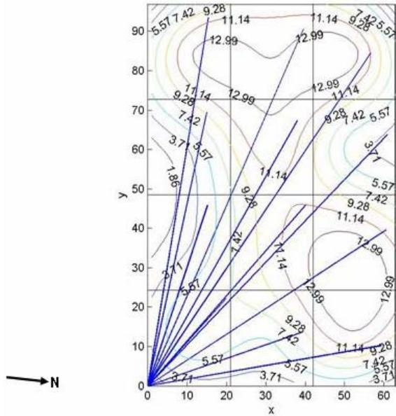
Figure B-3. Average Methane Surface Concentration Contour Map from the May 4 HRPM Survey of Area #2 (concentrations shown are in ppm above background)
