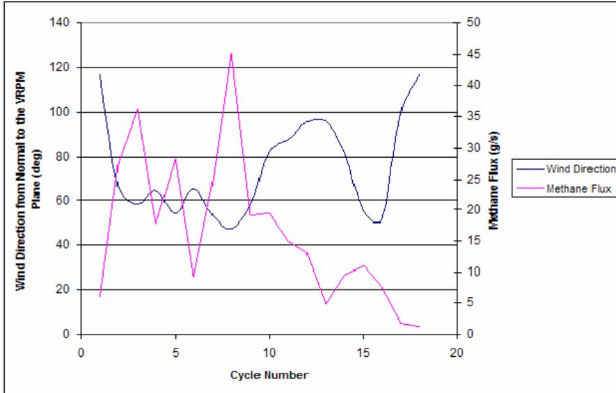
**Figure B-11. Time series of wind direction and methane flux values from the May 3 VRPM survey using the IMACC OP-FTIR**
