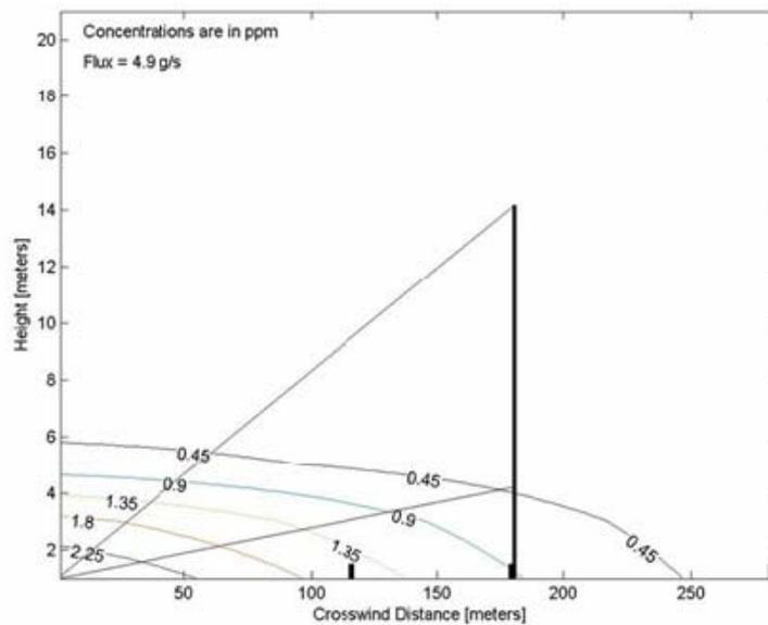
**Figure 4.** Example plume map generated using the VRPM method (concentrations shown in ppmv). The location of the vertical structure is shown by the solid black vertical line. The scanning ORS instrument is located in the bottom left-hand corner of the figure
