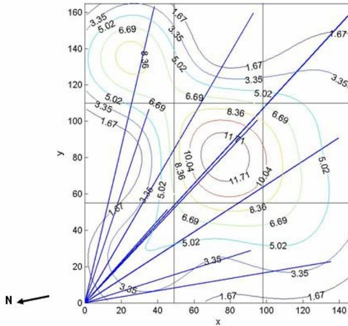
**Figure B-10. Average Methane Surface Concentration Contour Map from the May 5 HRPM Survey of Area #2 (concentrations shown are in ppm above background)**
