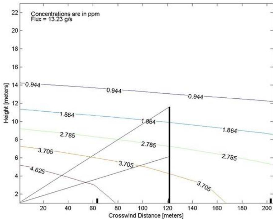
Figure C-5. Reconstructed methane plume map from the July 7 measurements.
