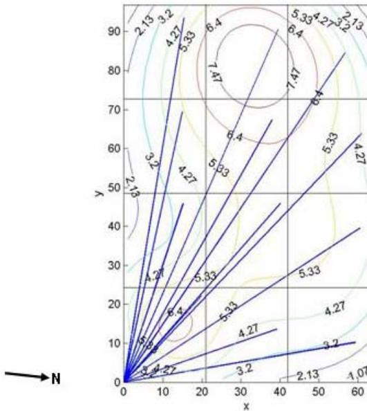
Figure B-4. Average Methane Surface Concentration Contour Map from the May 5 HRPM Survey of Area #2 (concentrations shown are in ppm above background)
