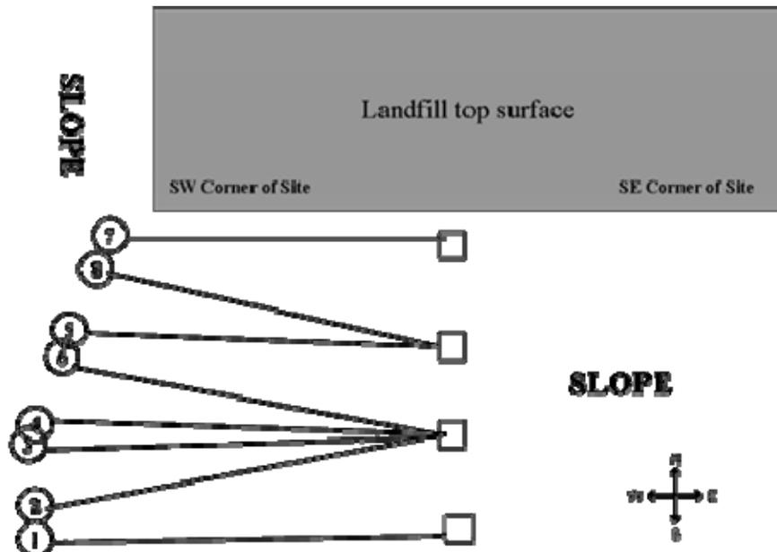
**Figure 18. Schematic of the OP-TDLAS configuration deployed along the southern slope of the Colorado Springs site**
