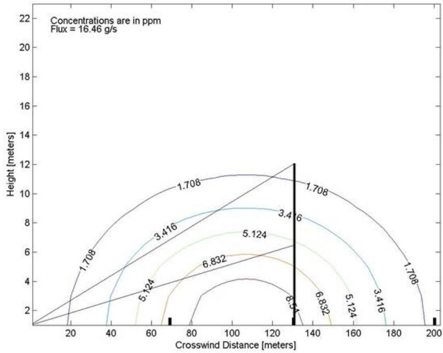
Figure C-1. Reconstructed Methane Plume Map from the June 19 Measurements
