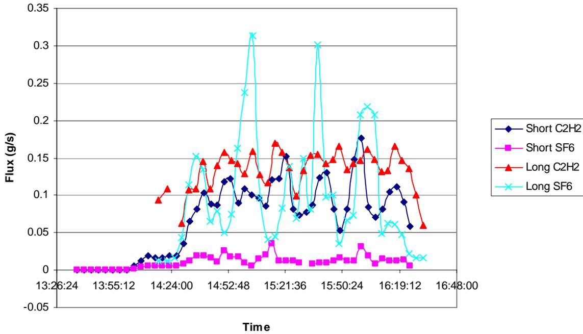
**Figure 26. Time series of acetylene and sulfur hexafluoride flux values from the 60 meter release survey**
