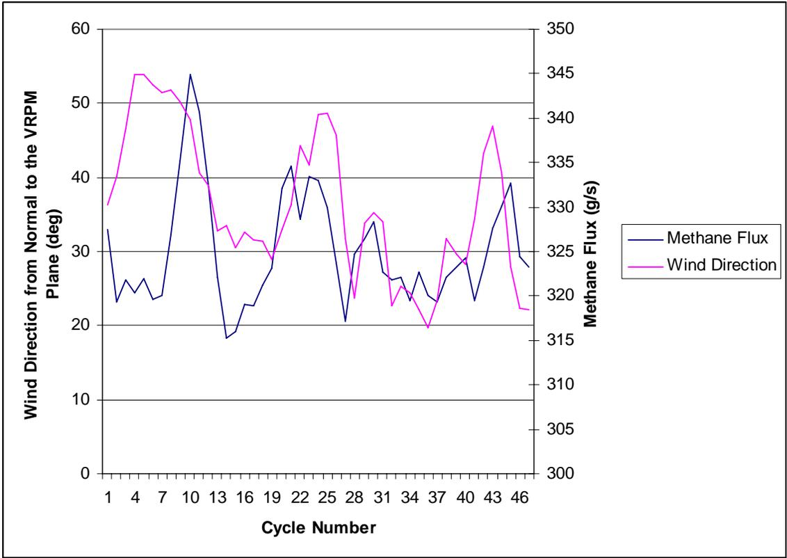
Figure C-4. Time series of wind direction and methane flux values from the July 5 VRPM survey.
