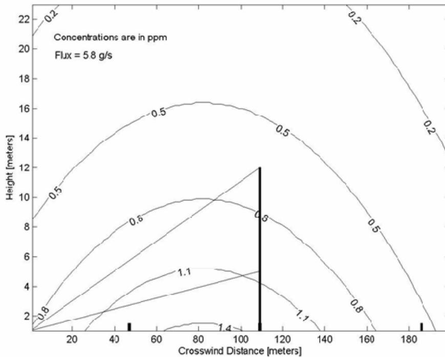
**Figure 13. Reconstructed methane plume map from the VRPM survey of the Somersworth site (concentrations shown in ppmv). The location of the vertical structure is shown by the solid black vertical line. The scanning ORS instrument is located in the bottom left-hand corner of the figure**
