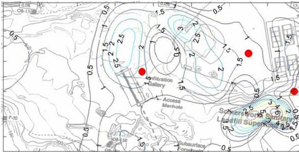
**Figure 12. Surface methane concentration contours (in ppmv) overlaid on the map of the Somersworth Superfund Landfill**
