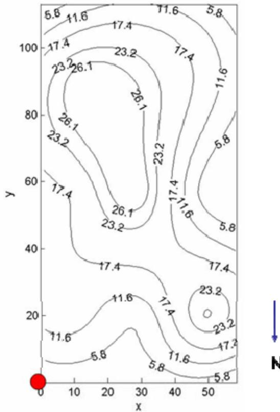
**Figure 2. Example surface methane concentration contour map generated using the HRPM method (concentrations shown in ppmv)**
