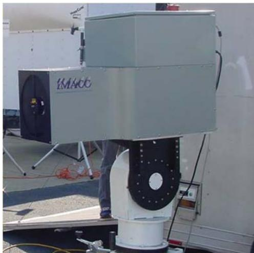
**Figure 7. IMACC OP-FTIR instrument and scanner**
