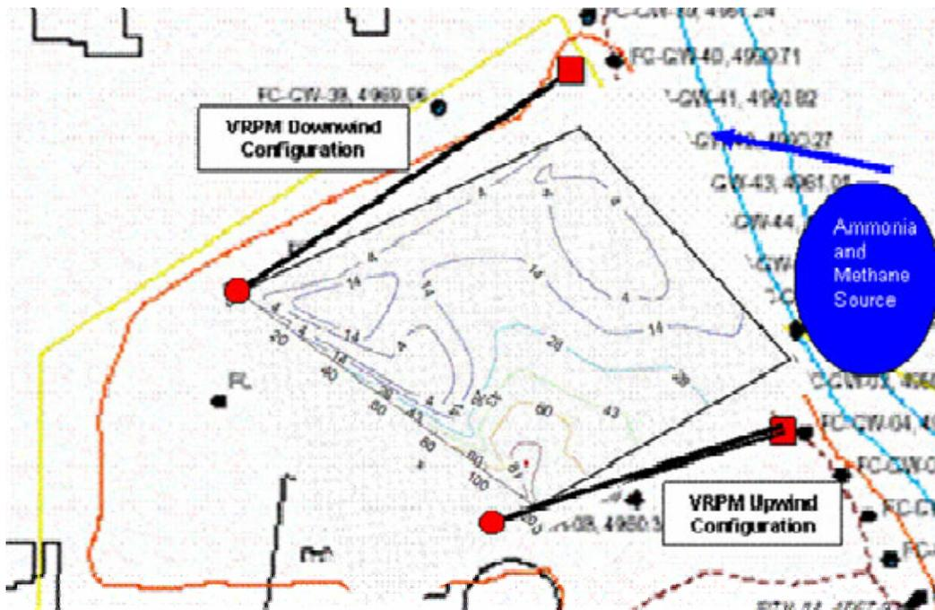
Figure 14. Summary map from the Fort Collins, CO site showing the surface gasoline concentration contour map (concentration shown in ppbv), and suspected source location of the measured methane and ammonia
