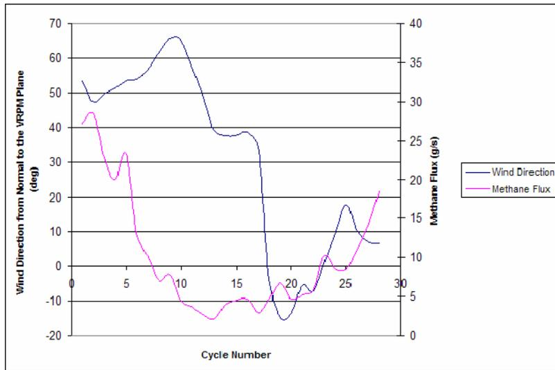
**Figure B-12. Time series of wind direction and methane flux values from the May 3 VRPM survey using the Unisearch OP-TDLAS**
