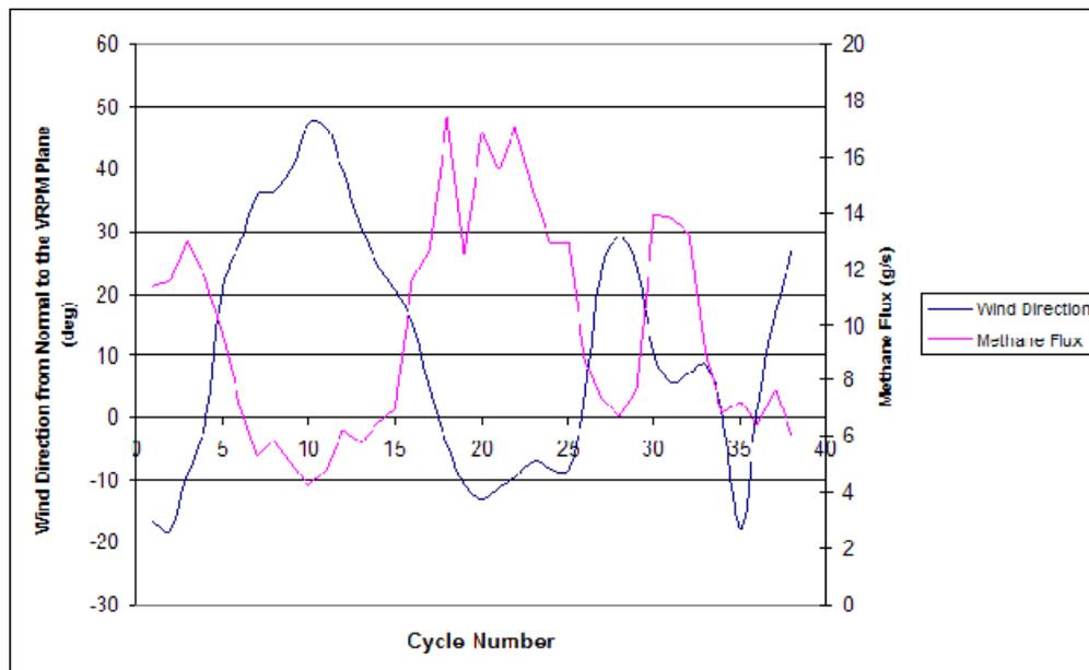
**Figure B-5. Time series of wind direction and methane flux values from the May 4 VRPM survey of Survey Area #2 using the IMACC OP-FTIR**
