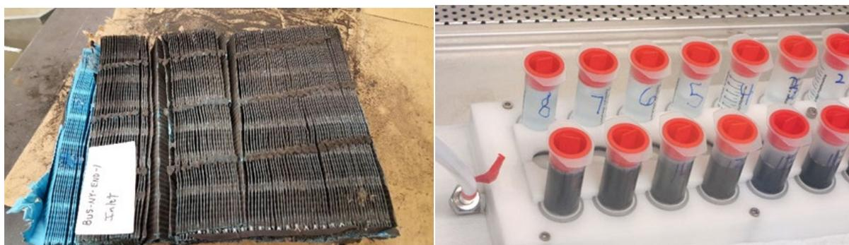
**Figure 29. Bus Engine End-of-Service Life Filter Deconstructed Prior to Spore Recovery (left) and Suspension After Recovered from Bus Engine Filters New (unused) in Top Row and End-of-Service Life in Bottom Row of RV-PCR Vacuum Manifold**
