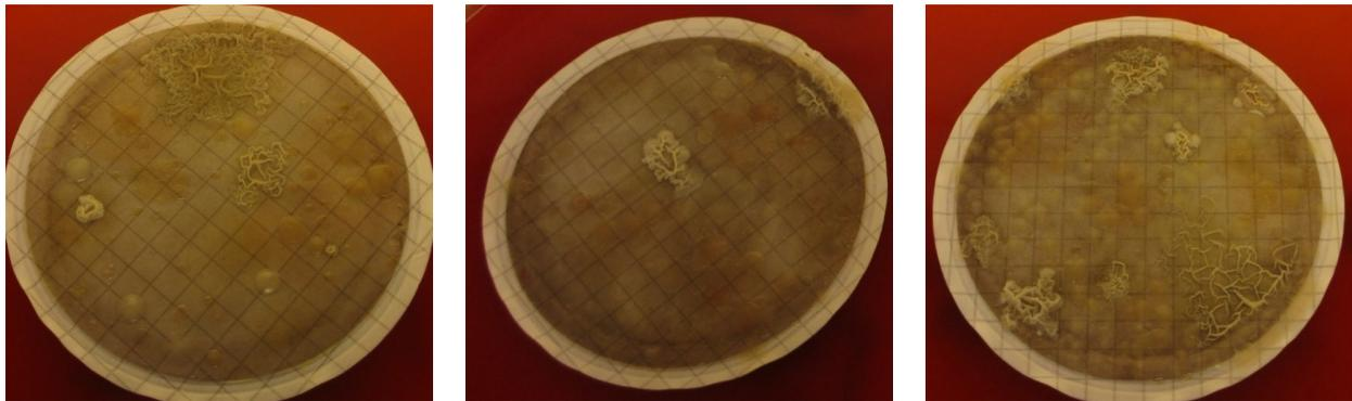
**Figure 24. Subway Rolling Stock End-of-Service Filter Spiked with 30, 300, or 3,000 Spores (from left to right, respectively)**
